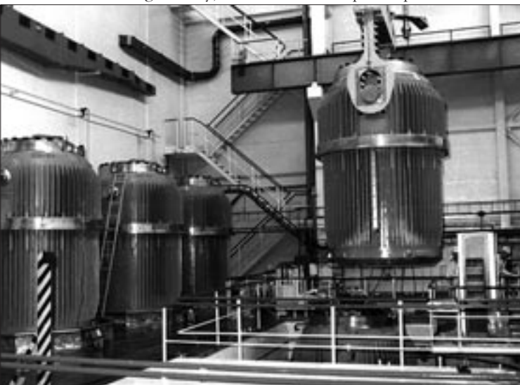
Containers of spent nuclear fuel in interim spent fuel storage facility, Bohunice nuclear power plant.
