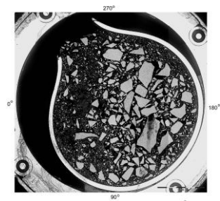
Figure 5 – Cross-section showing fuel relocation. Filling ratio 38%
