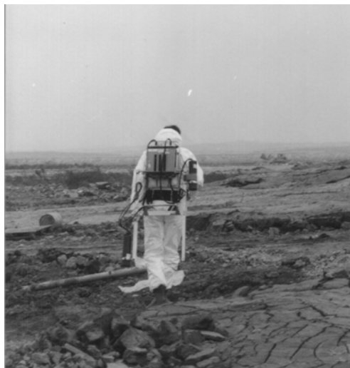
Figure 8. Spanish scintillation device for soil measurements
