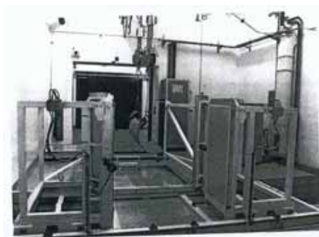
Figure 7. Bench for low level Control for beta-gamma emitters Plastic scintillators for Gross gamma counting
