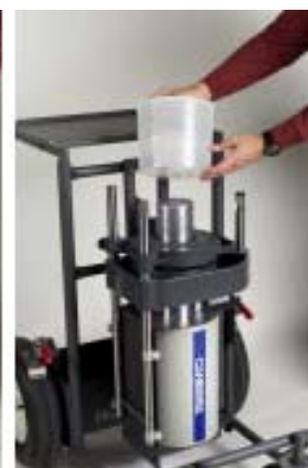
Figure 4.4 Can also count large samples in Marinelli beakers
