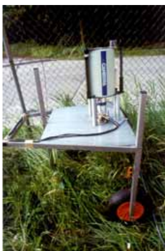
Figure 10. Release measurements for sites and buildings Collimated in situ gamma spectrometry – High purity Germanium
