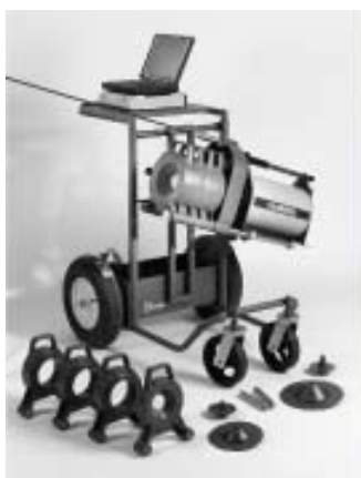
Figure 4.1 The ISOCS detector, cart, and shield components
