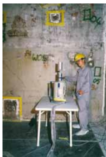
Figure 10. Release measurements for sites and buildings Collimated in situ gamma spectrometry – High purity Germanium
