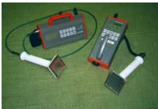
Figure 9. Portable ratemeters for surface measurements – Belgoprocess
