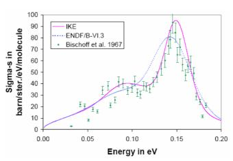
Incident neutron energy = 154 meV, scattering angle  $\theta = 60^{\circ}$ ). The figure is taken from the INDC report [72].
