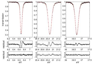
At room temperature or higher, Doppler-broadened cross-sections reconstructed from the resonance parameters using either the CLM or the usual free-gas-at-ambient-temperature method, will be indistinguishable. However, the reduced capture resulting from the low-temperature CLM fitting is still significant.
