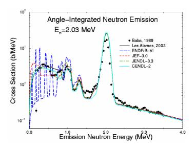
As displayed in Figure 9, the new evaluation features a softer inelastic secondary neutron spectrum compared with the previous one of ENDF/B-VI.8 or JEF-2.2. The influence of these new data on the smaller thermal benchmarks was found to be significant, increasing  $k_{eff}$  by reducing the neutron leakage, as explained in Section 5.
