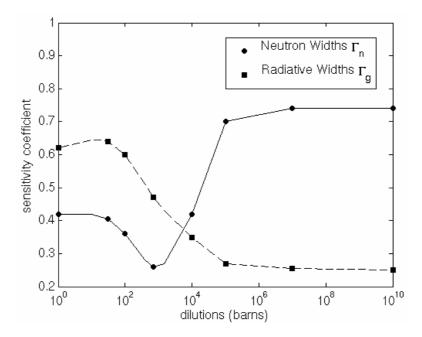
This figure shows the high sensitivity of the capture SRI to  $\Gamma\gamma$  in the dilution range typical of LWR (20-100 b)
