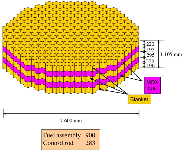
**Figure 12. Fuel assembly design of large-scale reduced-moderation water reactor (RMWR)**
