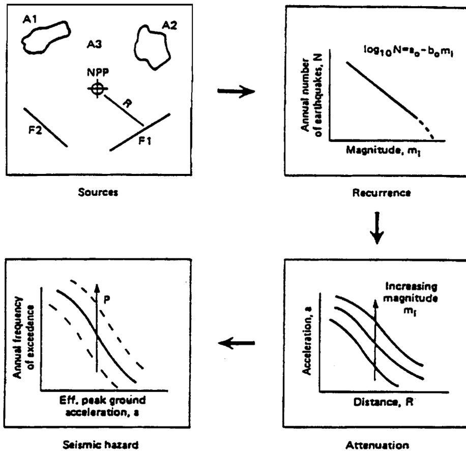
**Steps to Evaluate the Frequency of Exceedance of Ground Motion from Earthquakes**
