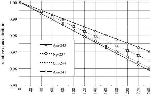
Figure 3 Evolution of selected MAs in the fast flux positions in Myrrha, with  $\phi$ >1.0 MeV = 1.0×10<sup>15</sup> n/cm<sup>2</sup>.s
