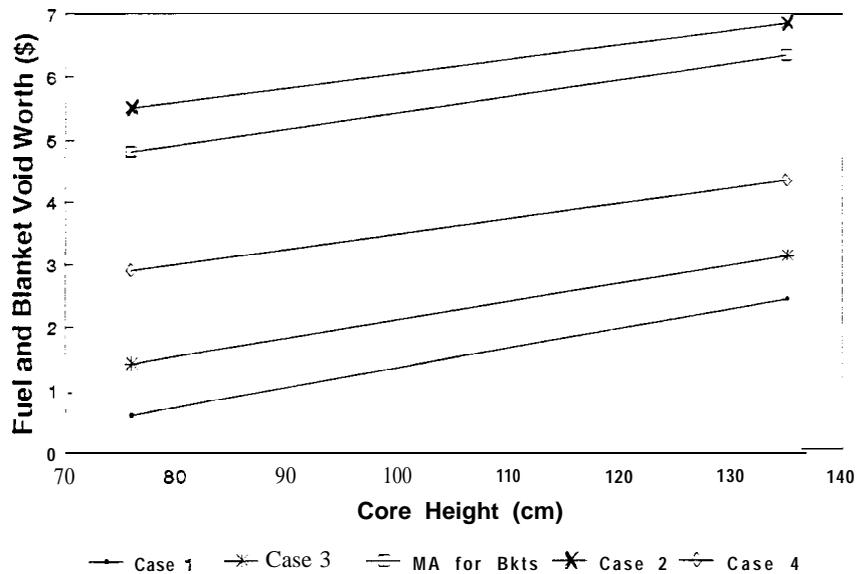
Fig. 2. Sodium Void Worth for Heterogeneous Core.
