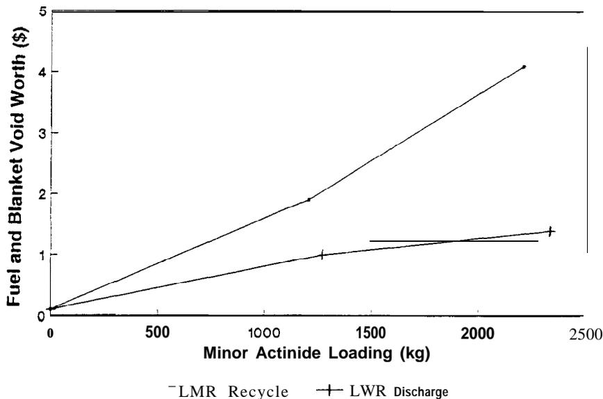
Fig. 4. Minor Actinide Loading Effect on NA Void.
