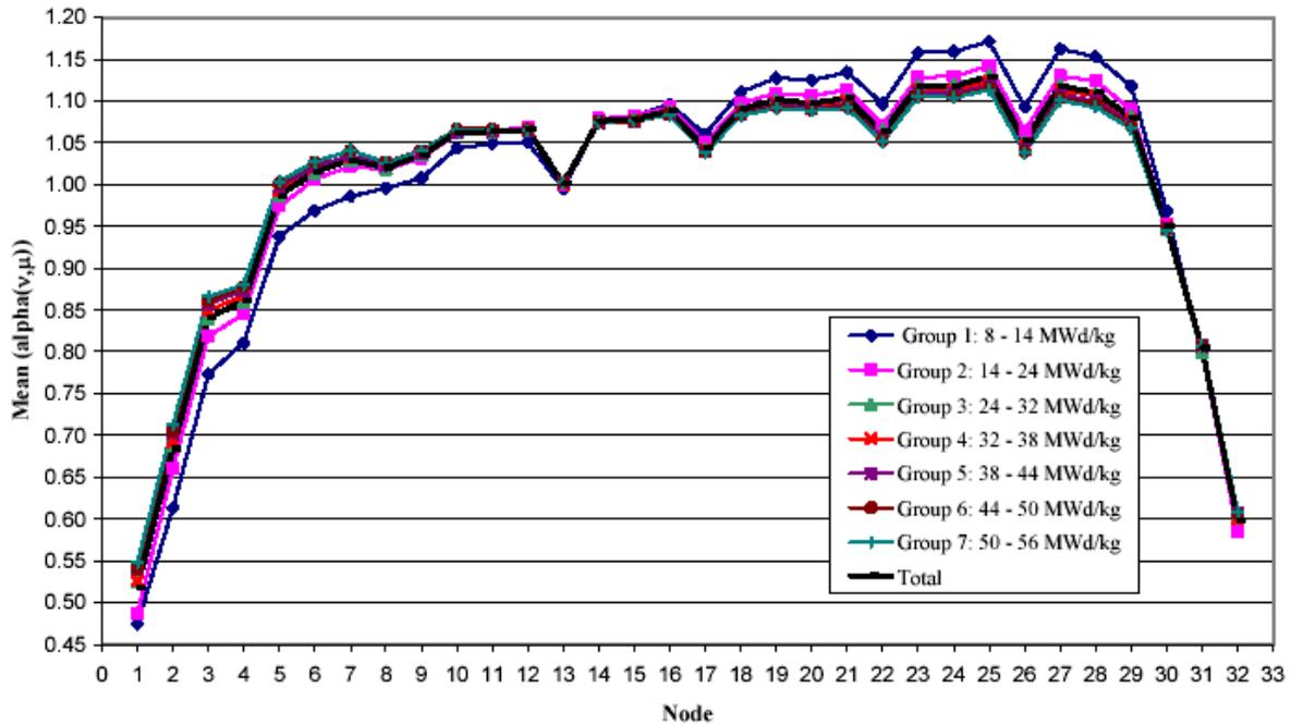
**Figure 2:** Evaluation of the axial burnup profiles from Ref. [6]: Averages  $\alpha_{v\mu}$  for the burnup groups into which the normalized burnup profiles were grouped according to their average burnup values
