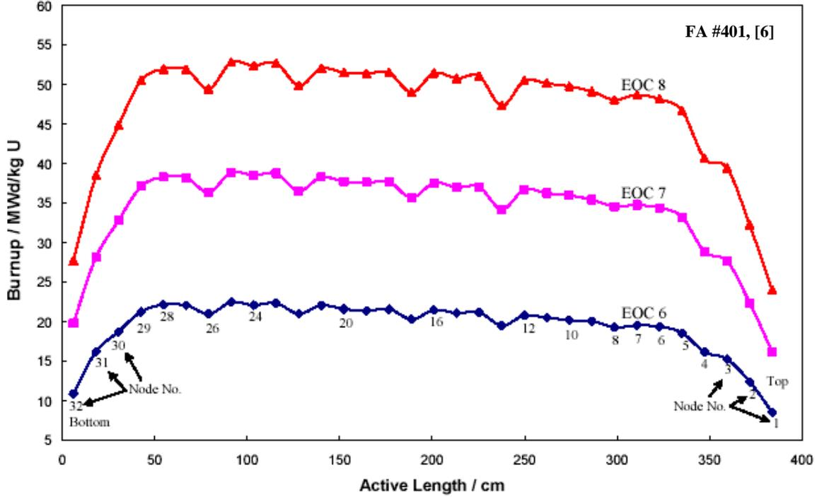
**Figure 1:** Three typical PWR axial burnup profiles obtained for one and the same fuel assembly in three consecutive cycles [6]. These profiles are visibly asymmetric, and the positions of the spacer grids within the active zone are clearly seen.
