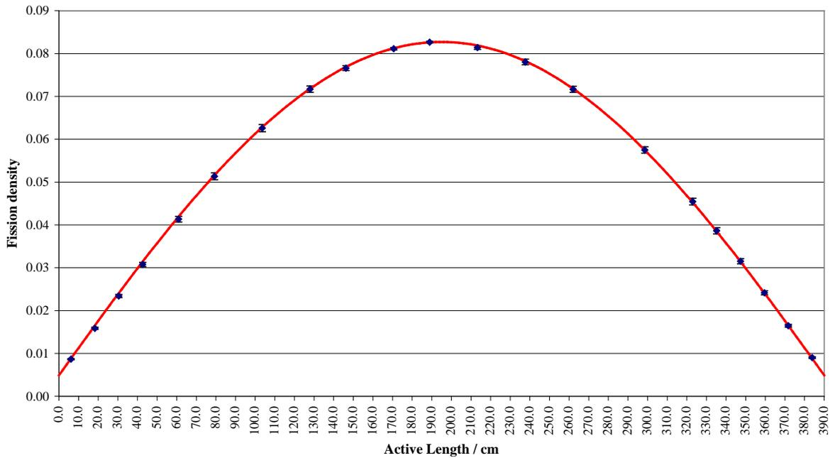
**Figure 10:** Non-normalized axial fission density distribution typical of uniform burnup distributions
