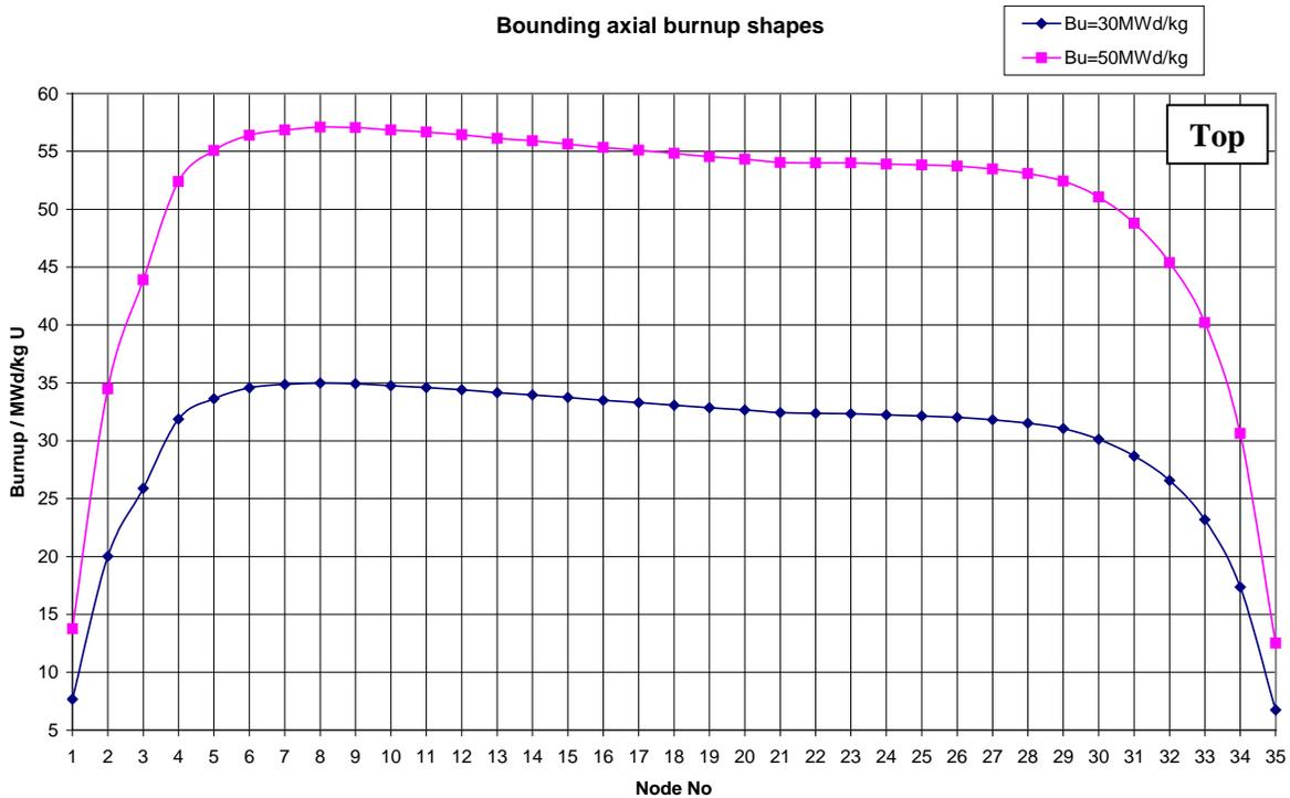
Figure 12: Axial burnup profiles chosen for the Phase II-E benchmark program
