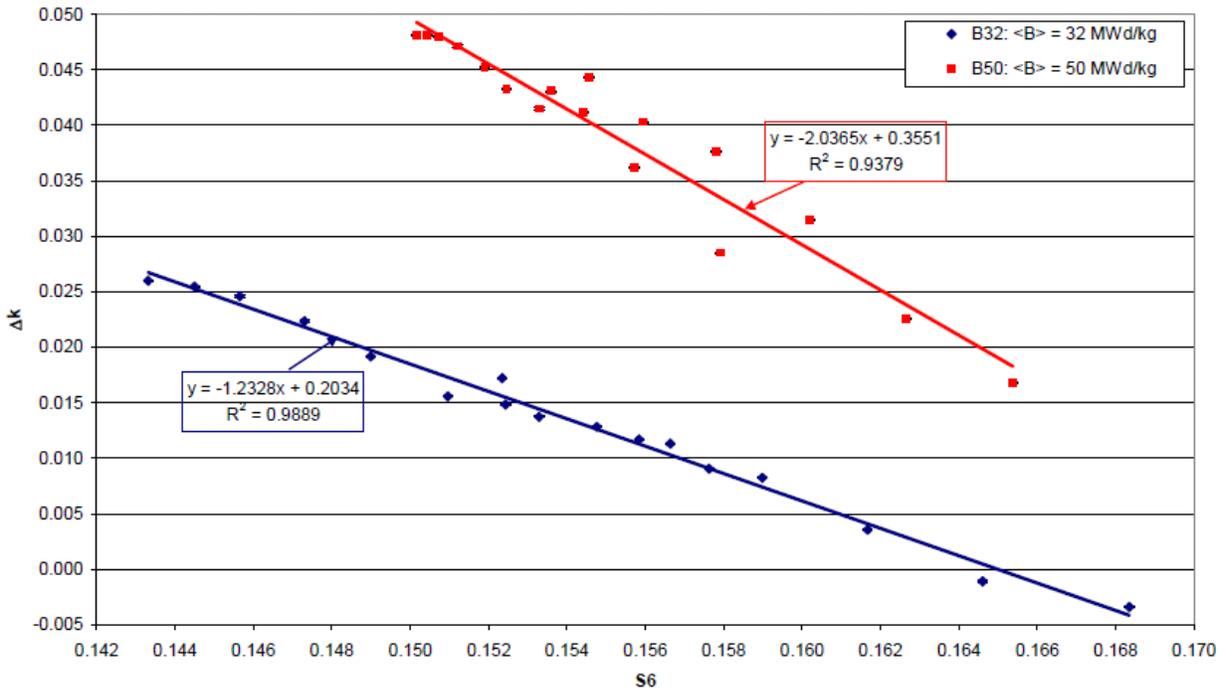
**Figure 6:** Regression analysis of the observed end effect values  $\Delta k_{ee}(B32)$  and  $\Delta k_{ee}(B50)$  as a function of the top end parameter  $S6$
