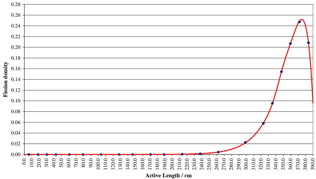
*Figure 11: Comparison of the non-normalized fission density distributions obtained for the reference profiles B32A222222 and B50A222222*
