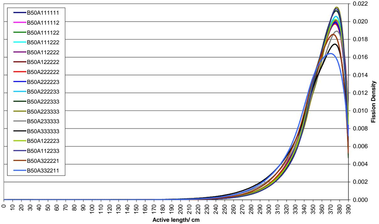
**Figure 8:** Normalized fission density distributions obtained for the profiles with 50 MWd/kg U average burnup
