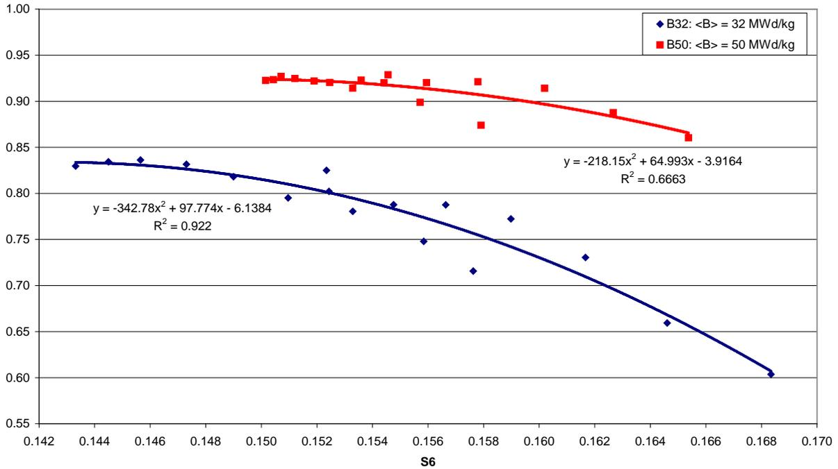
**Figure 9:** Regression analysis of the C6 values obtained for the Phase II-C axial burnup profiles
