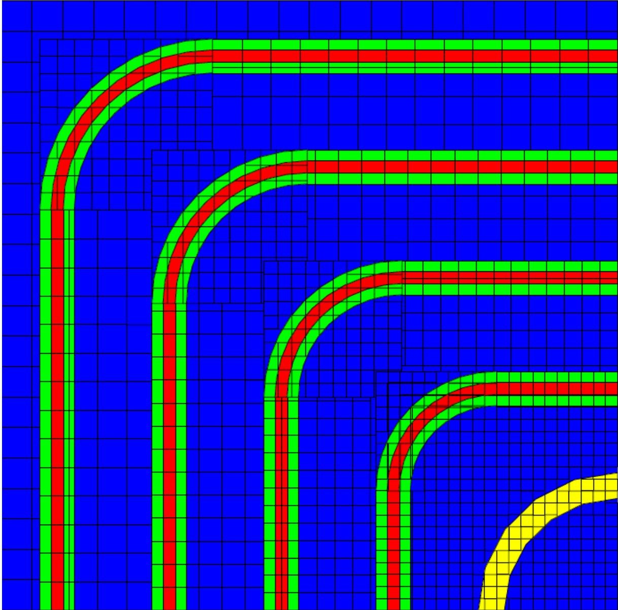
Fig.1. Quarter of horizontal section of IRT-2M four-tube fuel assembly (TRITON output)
