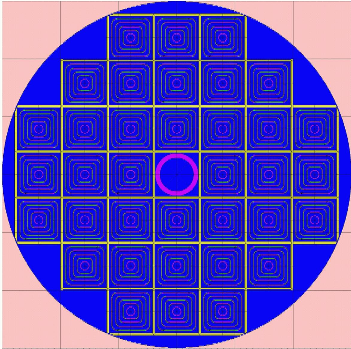
Fig.4. Horizontal section of VPVR cask basket loaded with IRT-2M fuel assemblies with initial enrichment of 36 wt.%  $^{235}\text{U}$  , ATABOR intervening shielding plates (MCNP output)
