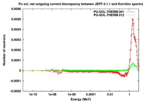
FIG. 3. Fissile zone outgoing net current discrepancy between JEFF-3.1.1 and Kornilov spectra calculations.
