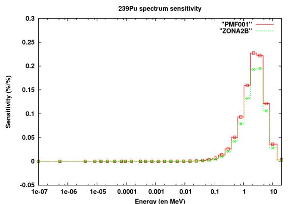
FIG. 2.  $k_{eff}$  sensitivities on spectrum for ZONA2B and PU-MET-FAST 001 fast flux spectrum experiments.
