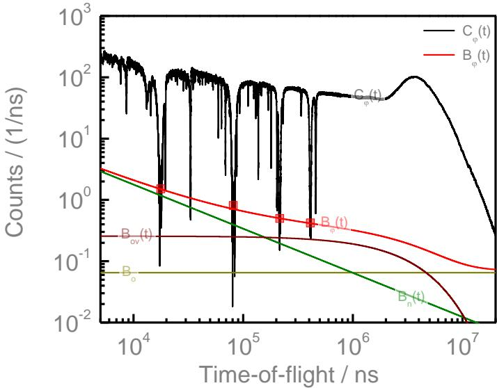
$$Y_{\text{exp}} = N \frac{C'_w - B'_w}{C'_\phi - B'_\phi} Y_\phi$$
