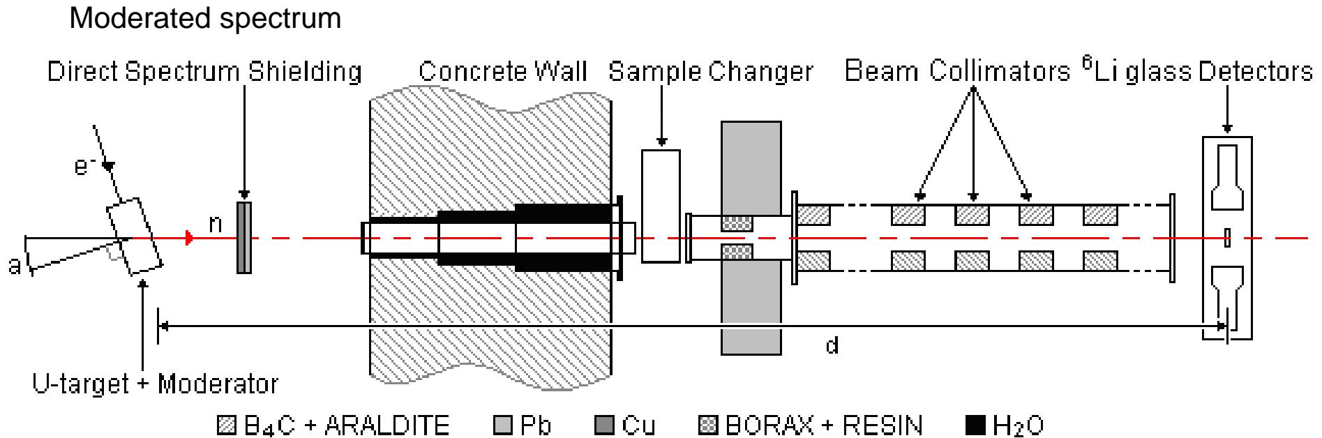
$$T_{\text{exp}} = \frac{C_{\text{in}} - B_{\text{in}}}{C_{\text{out}} - B_{\text{out}}} \leftrightarrow e^{-n\sigma_{\text{tot}}}$$
