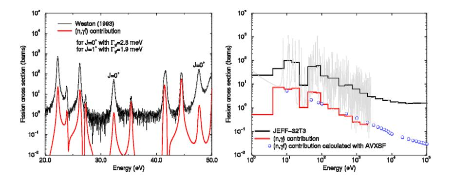
The smallest resonances with  $J^{\pi}=1^{+}$  are dominated by the (n, $\gamma$ f) process
