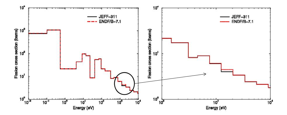
Modification of  $\alpha$ (Pu239) in JEFF-311 to improve the reactivity temperature coefficient (RTC) in EOLE experiments, cold conditions 20-80°C (JEF/DOC-1158)
