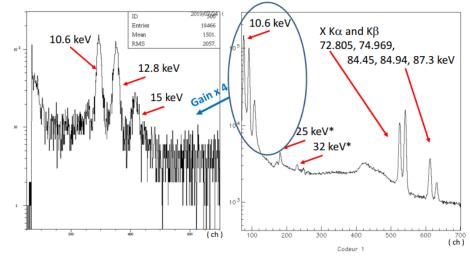
After several investigations, the collaboration has now a suitable detector for the observation of electrons coming from internal conversion process in actinides. Tests with 238U sample are planned as soon as it will be possible to go on site.
