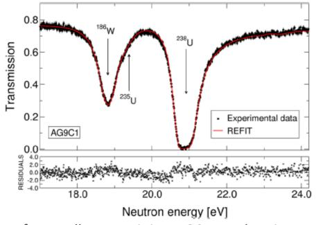
NRTA for a pellet containing UO2+Ag, showing a significant amount of W not reported in the specifications
