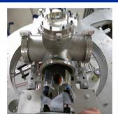
DSSSD setup with back-toback 14N and 35Cl samples Additional runs with dummy (Al backing) and a 10B reference
