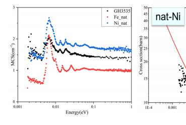
➤ It can be observed that the energy positions of Bragg-edges, and the Miller indices corresponding to the micro crystal structure (FCC) of the sample GH3535 are shown for each distinguishable Bragg-edge.
