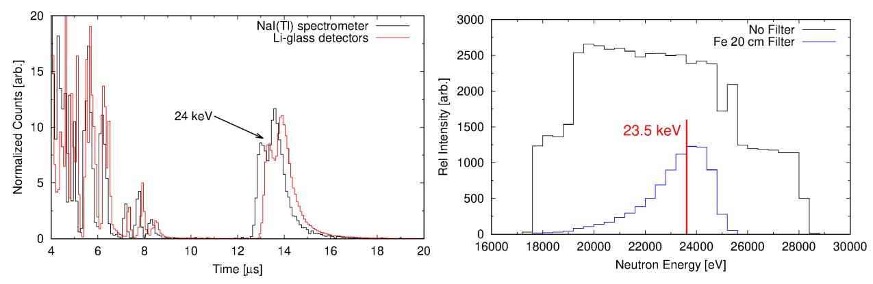
Filtered neutron beam through **20 cm of Fe** measured by **Li-glass detectors** and a **Nal(TI) spectrometer** (with B sample).
