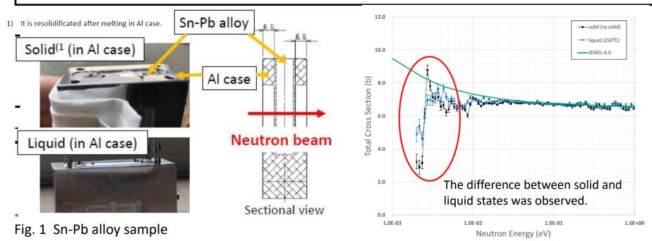
Transmission neutrons were measured by a <sup>6</sup>Li-glass detector. The flight length was 12.1 m.
