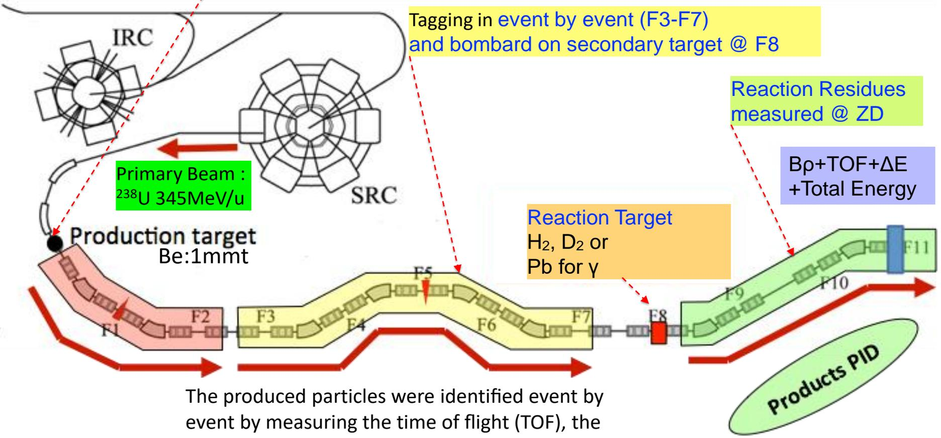
The produced particles were identified event by event by measuring the time of flight (TOF), the magnetic rigidity (Bp), and the energy loss ( $\Delta E$ )
