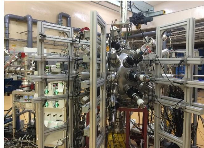
Array of 33 liquid scintillators (d5"x t2") around the fission chamber ( Planning to add 12 detectors. )
