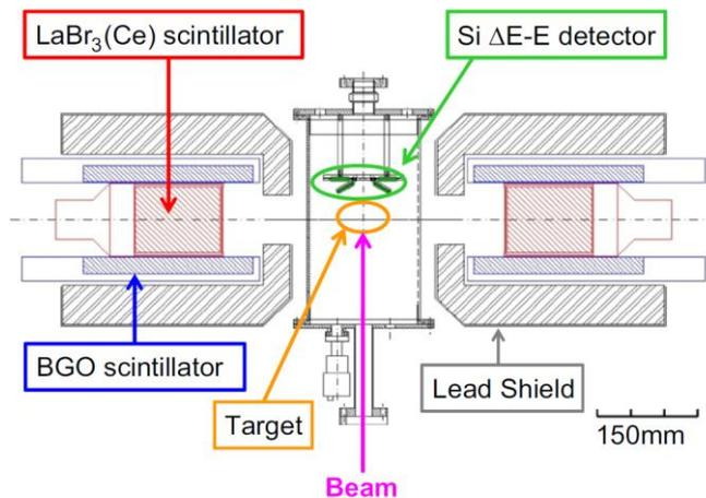
Detector setup for the surrogate capture measurement.
