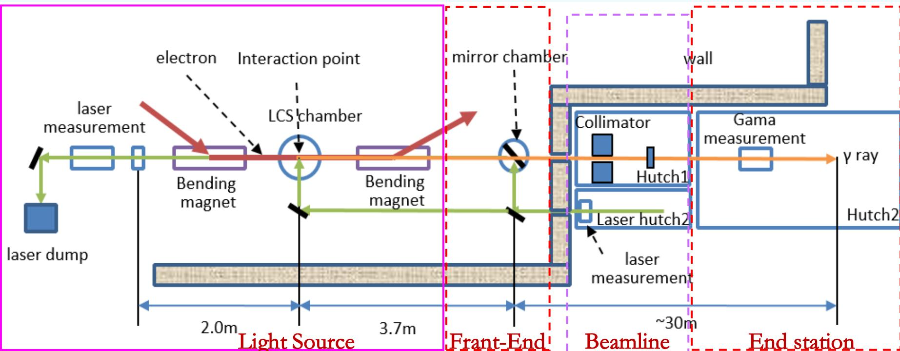
(1) Light source: electron, laser, LCS chamber(slanting mode), mirror chamber(back scattering).
