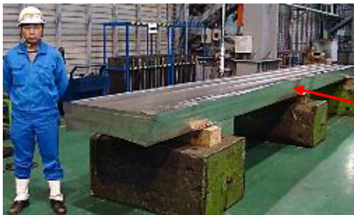
JJ1 large forging (860mm width, 250mm thickness, 7,600mm length)
