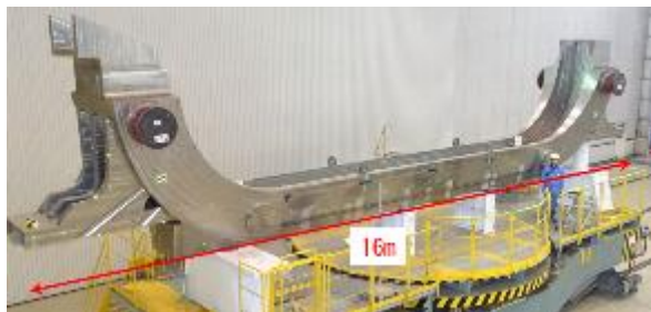
AU completed welding
