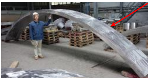
C3 material being longest forging (910mm width, 133mm thickness, 9200mm length)
