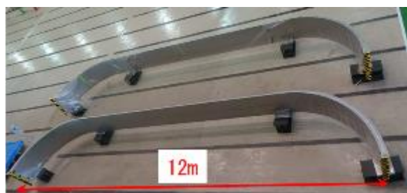
AP completed welding
