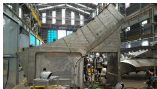
Part of BU under welding
