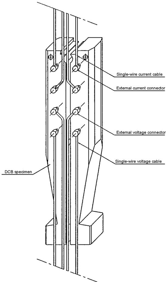
Instrumented pre-irradiated DCB specimen
