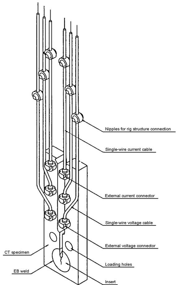
Instrumented CT specimen with pre-irradiated circular insert
