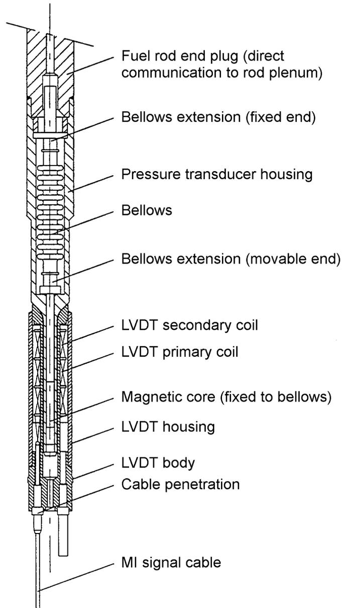
**Figure 2. Re-instrumentation of pre-irradiated fuel rods**
