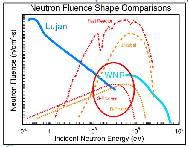
Redesign spallation moderation target to increase fluence in intermediate energy region
