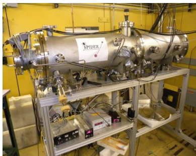
SPIDER 2E-2V for fission fragment yield measurements
