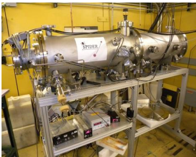
SPIDER 2E-2V for fission fragment yield measurements
