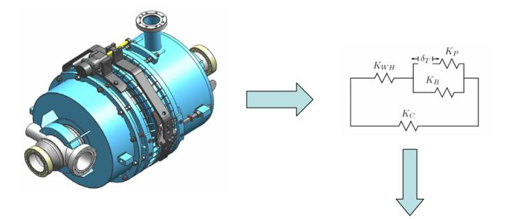
$1/K_{ext} = 1/K_{H} + 1/K_{T} + 1/K_{W} + 1/(2K_{P}) \rightarrow K_{ext} = 9.2 > 9 \text{ kN/mm}$
