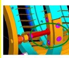
2 piezo elements, stroke depends on their length. For L = 40 mm we expect more than  $2\mu$ m of displacement (> 700 Hz) maximum elongation of approximately 1.3 mm that corresponds to a cavity stretching of 1.2 mm ( $\cong$ 400 kHz)
