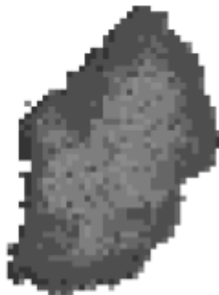
Figure 3. \mu -XANES imaging of a particle collected to the north of the Chernobyl reactor, released during the reactor fire. The particle has a \text{UO}_2 core surrounded by an oxidised \text{U}_2\text{O}_5/\text{U}_3\text{O}_8 surface layers.
