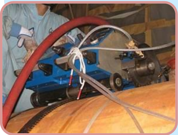
Orbital pipe cutting machine
