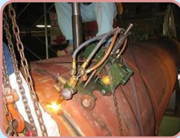
Automatic gas cutting machine (self-propelled)
