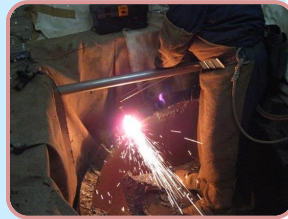
Gasoline oxygen cutting (manual)
