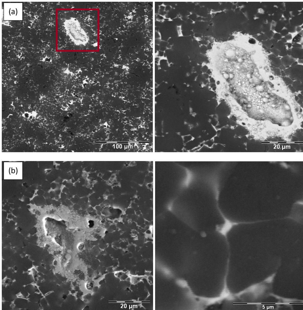
irradiation which cannot be dissolved in standard reprocessing conditions. Another sample was thus dissolved by using a boiling 4 M  $\text{HNO}_3$  acid solution including 0.1 M HF in order to achieve full dissolution for chemical analysis. From these analyses, Am transmutation and fission rates could be determined: respectively 94 and 25 at.%. It should be noted that almost the same values were found by means of EPMA.
