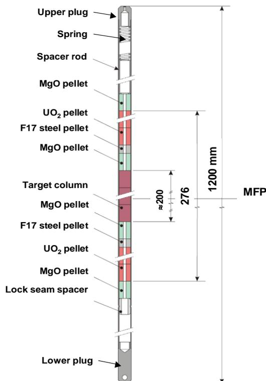
The ECRIX-H pin is placed in a specific carrier subassembly equipped with annular blocks of  $\text{CaHx}$  which act as a moderator. When combined with a high neutron flux in an FR, the increased cross-sections due to the slowed neutrons makes it possible to achieve high rate in minor actinide
