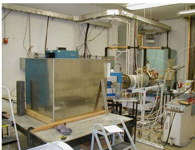
Figure 4. The 30-MeV Electron Linac. Peak performance is achieved at 25 MeV. In addition, peak power occurs at less than the maximum energy, so that the accelerator is currently operated at 20 to 25 MeV. The tank and stand are also visible.
