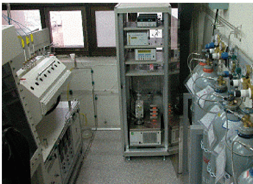
Figure 3. Gas system of the KAERI static corrosion facility
