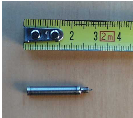
Figure 2. Photograph of a manufactured microscopic fission chamber (before connecting with a coaxial mineral insulator cable)
