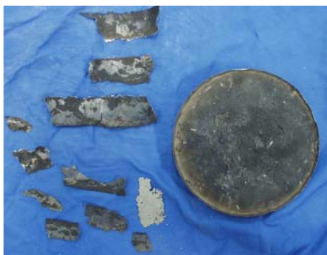
Figure 9. Heel ingot from the injection casting and the peeled off dross
