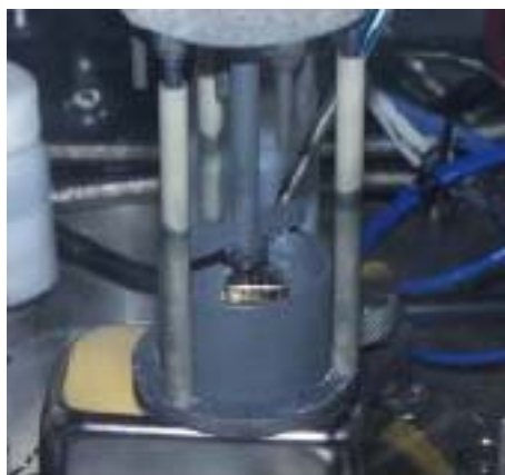
Figure 4. Liquid Cd cathode crucible and stirrer
