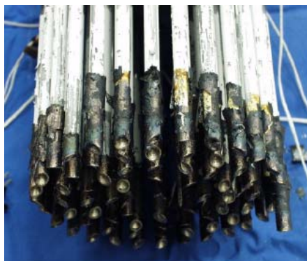
Figure 10. Fuel alloy adhesion at the bottom of the molds
