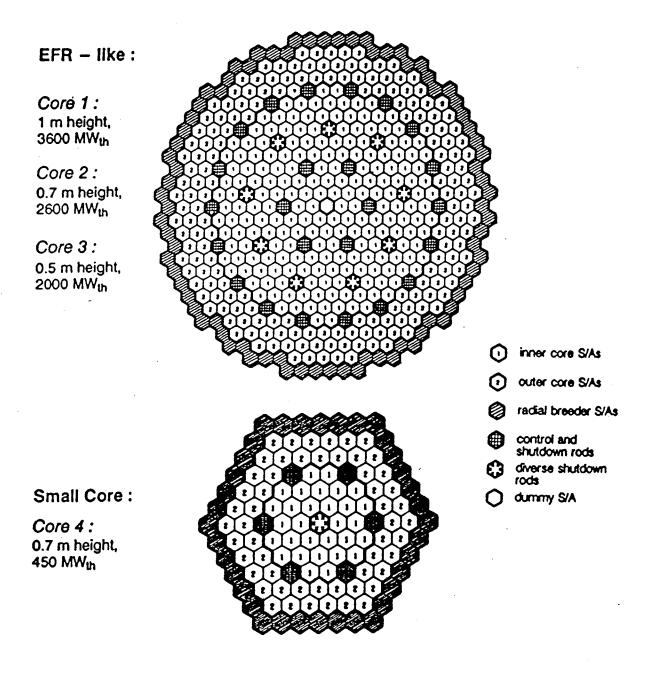
VG 3 : Core layouts with different core size
