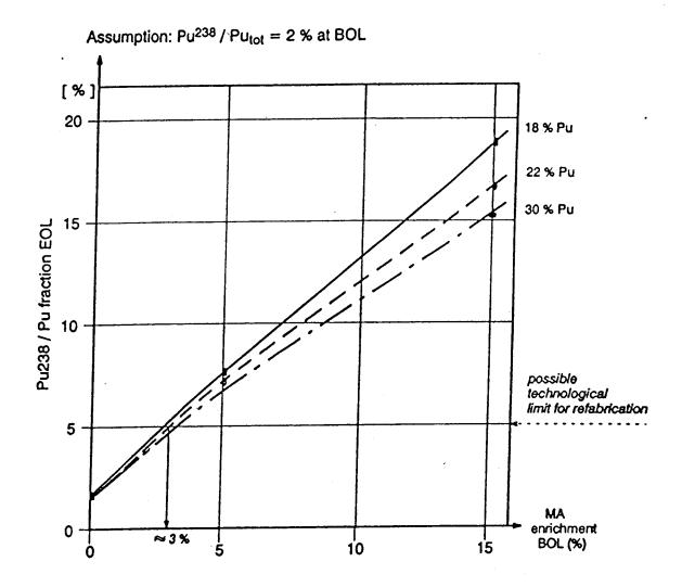
VG 6 : Pu238 generation in MA containing cores
