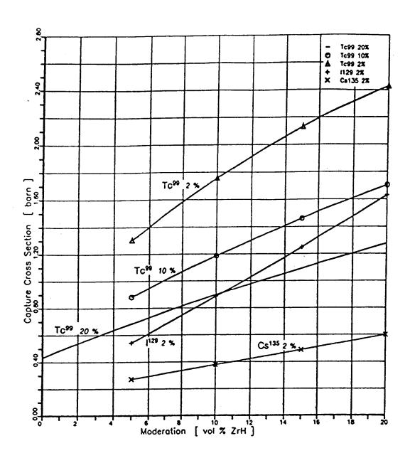
VG 8 : One–group capture cross–sections for Tc–99, I–129 and Cs–135 in dependence on moderator content
