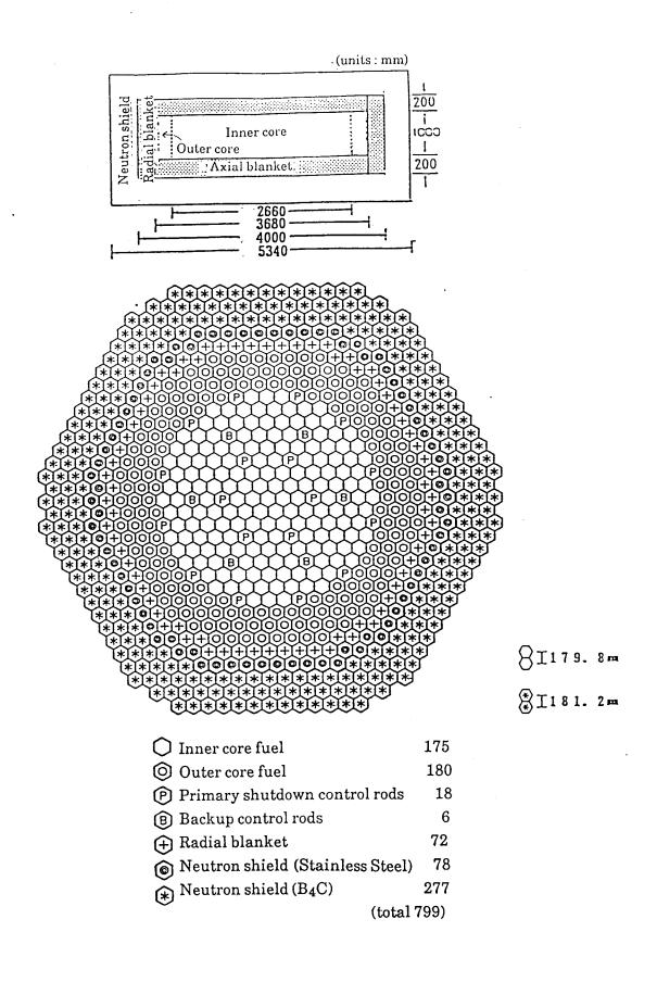
Fig. 1 Core layout of 1000MWe-class reference LMFBR
