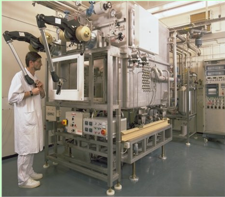
Figure 4.12: The stainless steel caisson for the pyro-processing installation at the Institute for Transuranium Elements, JRC Karlsruhe
