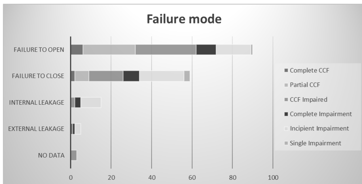
Figure 3.3. Distribution of failure modes and event severities
