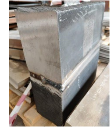
Welding of the qualification sample from rolled sheets
