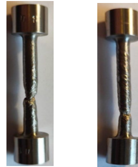
4C57 alloy samples after testing
