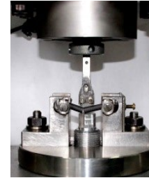
Testing of graphite samples, a capsule with samples prepared for irradiation
