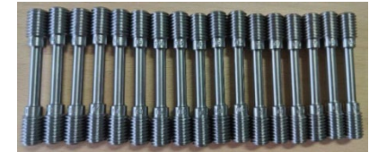
Samples of the welded joints after testing
