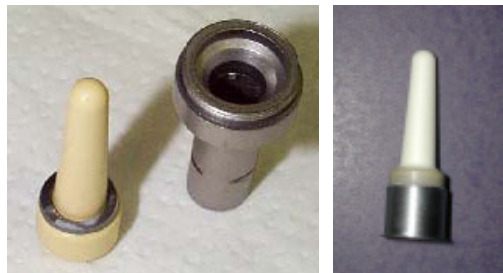
Figure 4.4.9. LANL ceramic element with the graph-lock gasket and the metallic sheath with the seating ring [Li, 2003] and the reactive braze bound [Ballinger, 2006]
