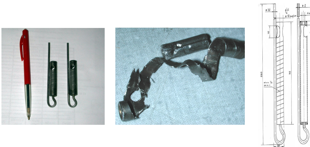
Figure 4.4.10. Scheme, view of the dip sampling system, which is then hooked to a stem and immersed throughout an air lock, as well as the resulting LBE sample
