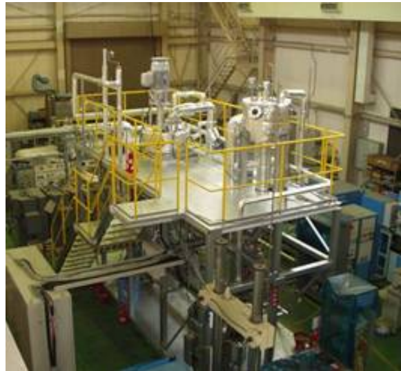
JLBL-3 for thermal-hydraulics of beam window
