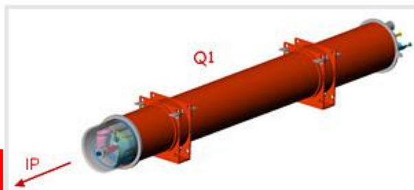
Q1 Quadrupole Magnet – CERN and Fermilab are working to identify repairs to the structures that hold the cold mass (blue) in place within the cryostat (orange) in each magnet of the triplet on either side of the LHC's four interaction points. The Q1 magnet of each triplet is the magnet closest to the interaction point (IP).
