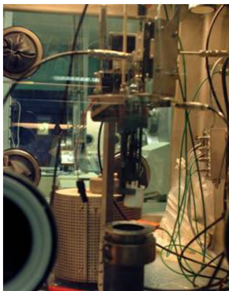
High Temperature Salt/Metal Contactor in glove-box (Atalante)
