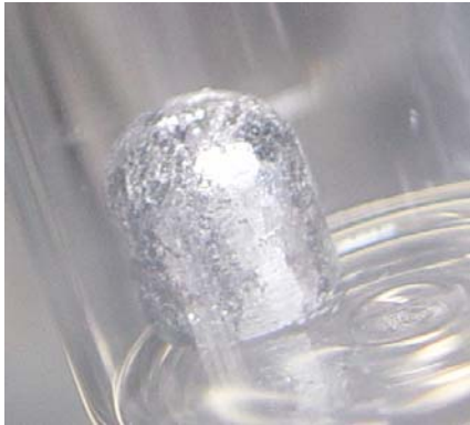
Appearance of (U,Pu,RE)-Cd alloy
