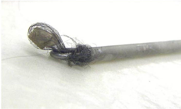
Appearance of (Pu,Zr)N anode used for the cyclic voltammetry and the potential controlled electrolysis
