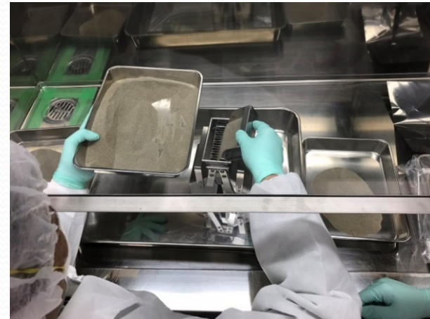
Division of sediment samples by the splitter. These samples were subsequently analyzed in parallel by laboratories in Japan and IAEA.
