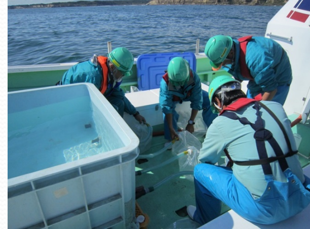
A large plastic container with valves was filled with surface seawater and sub-samples of 20L-plastic containers were filled from each valve.
