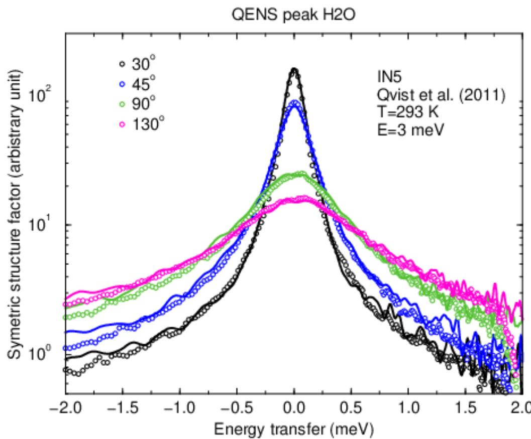
QENS and libration band of H<sub>2</sub>O measured with the IN5 and IN4 time-of-flight spectrometers of ILL
