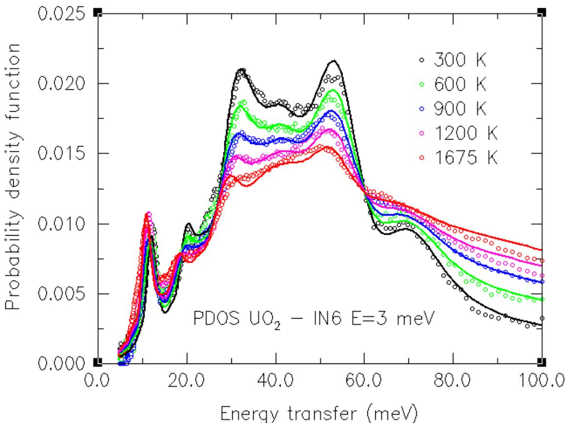
PDOS of UO<sub>2</sub> extracted from INS data measured with the IN6-SHARP time-of-flight spectrometer of ILL
