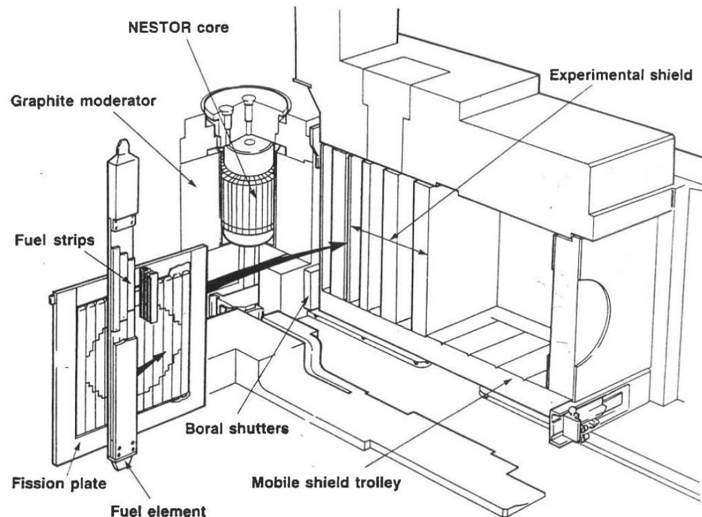
**NESTOR is a graphite-moderated water-cooled thermal reactor with a thermal power of 30 kW**
