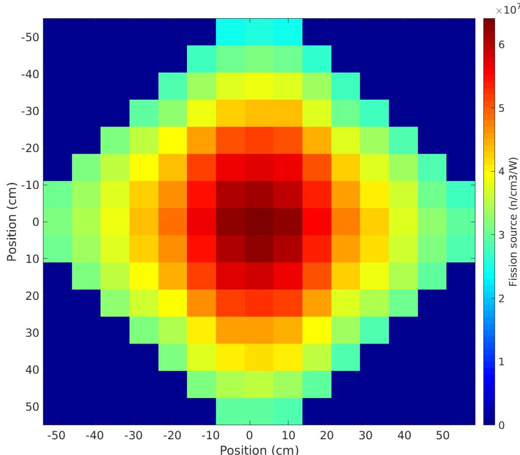
**Thermal neutrons leaking from the reactor induce fissions in this plate**
