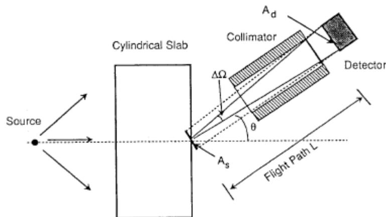
Fig. Diagram of FNS experiment
