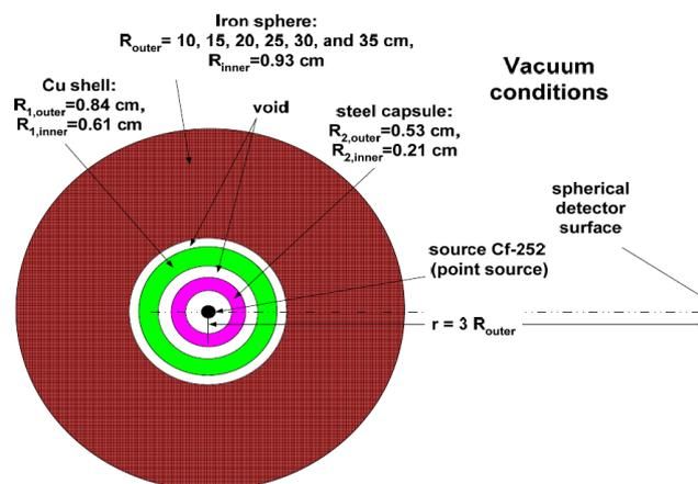
Fig. Diagram of ALARM-CF-FE-001 experiment
