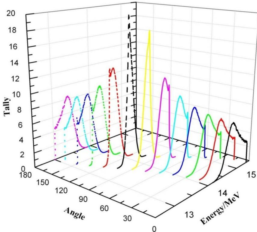
Fig.11 The angle dependent energy distribution of the source neutrons(by TARGET code)
