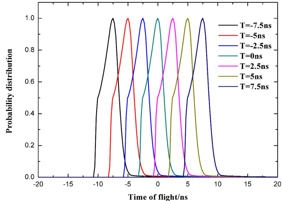
Fig.12 TOF spectra of neutron source at  $0^\circ$  and 8m with different generation time
