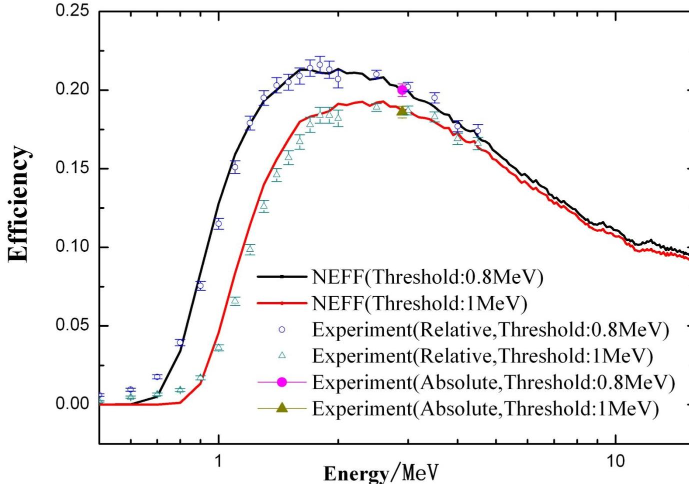
Fig.6 The detection efficiency with different thresholds
