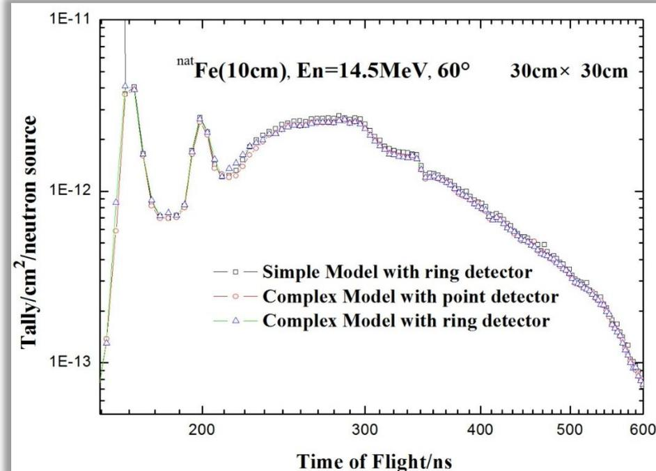
Fig.10 The simulation results from different models; Φ13cm(left), 30cm × 30cm(right)
