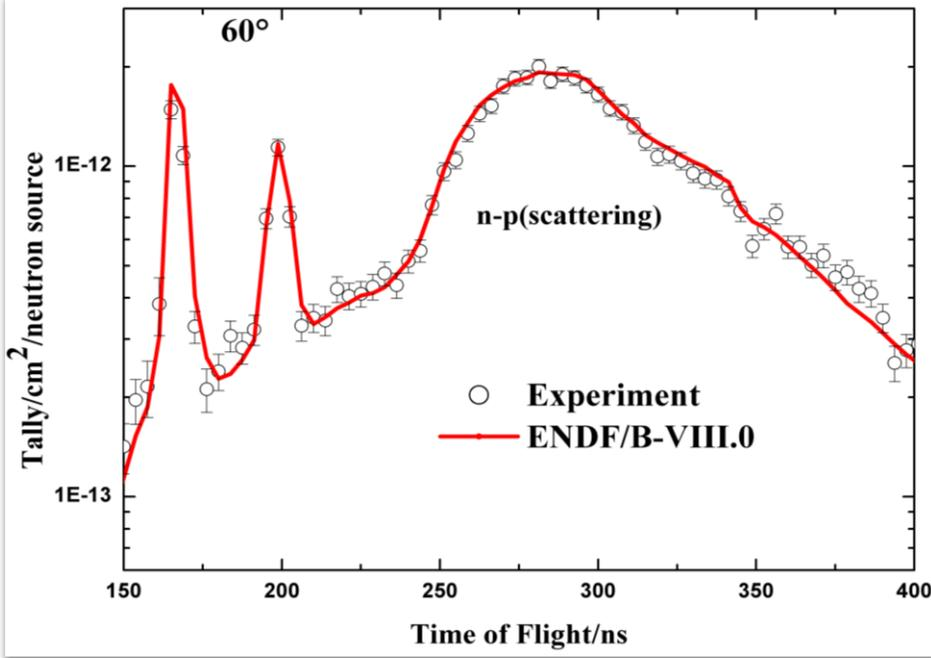
**Fig.7** Leakage neutron spectra from polyethylene sample of  $\Phi 13\text{cm} \times 6\text{cm}$  at  $60^\circ$
