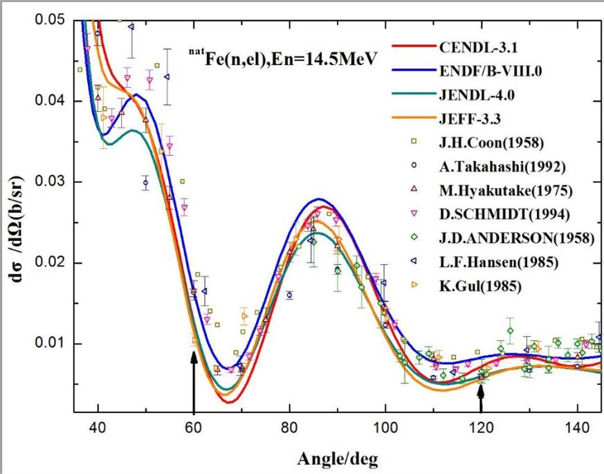
Fig.16 The angular distributions of the neutron elastic scattering
