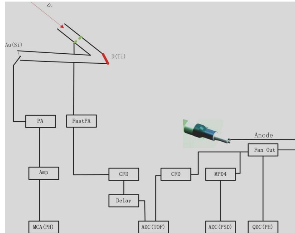
**Fig.4 Experimental arrangement for relative detection efficiency calibration**
