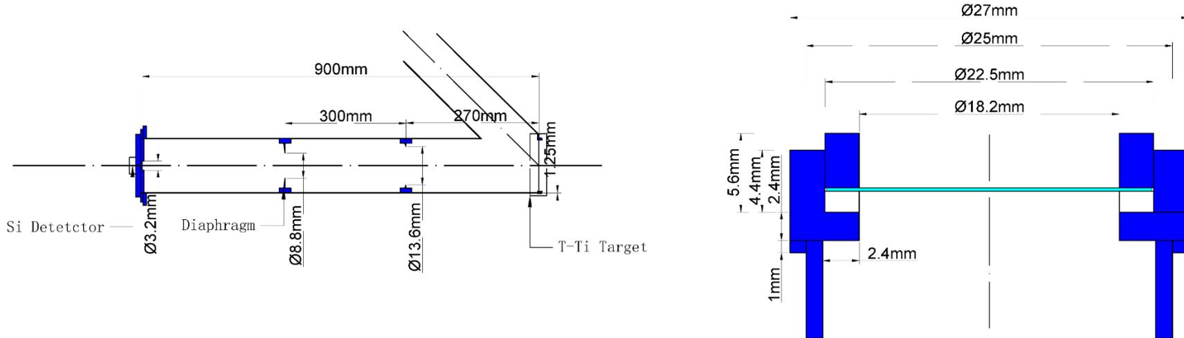
Fig. 2 The detailed dimensions with the T-Ti target
