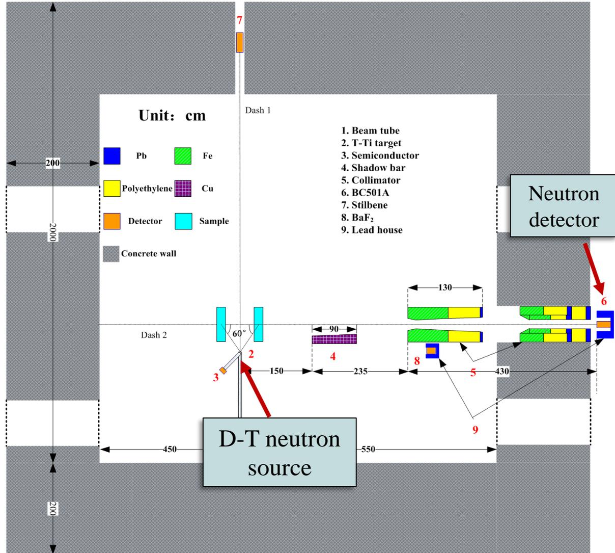
Measure the neutron leakage spectrum from slab samples for different angles by Time-of-Flight technique with a 14 MeV D-T neutron source
