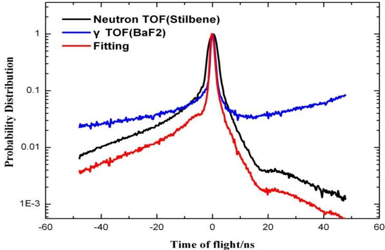
Fig.13 Comparison of the fitting result with the neutron spectrum and the  $\gamma$  spectrum
