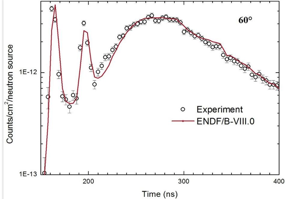
**Fig.8** Leakage neutron spectra from polyethylene sample of  $30\text{cm} \times 30\text{cm} \times 6\text{cm}$  at  $60^\circ$
