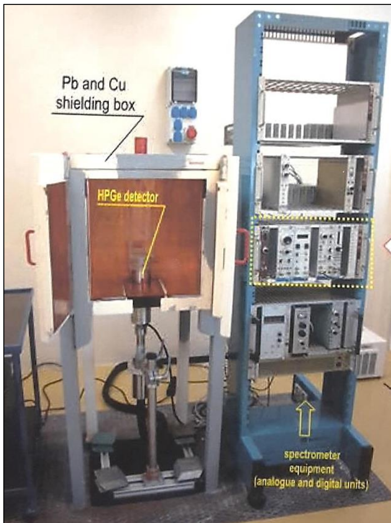
HPGe detector and spectrometer for AF and irradiated samples measurement SW - GENIE2000
