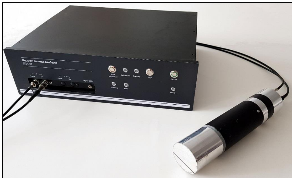
Digital spectrometer FD-13 with PSD Stilbene Detector with Photomultiplier
