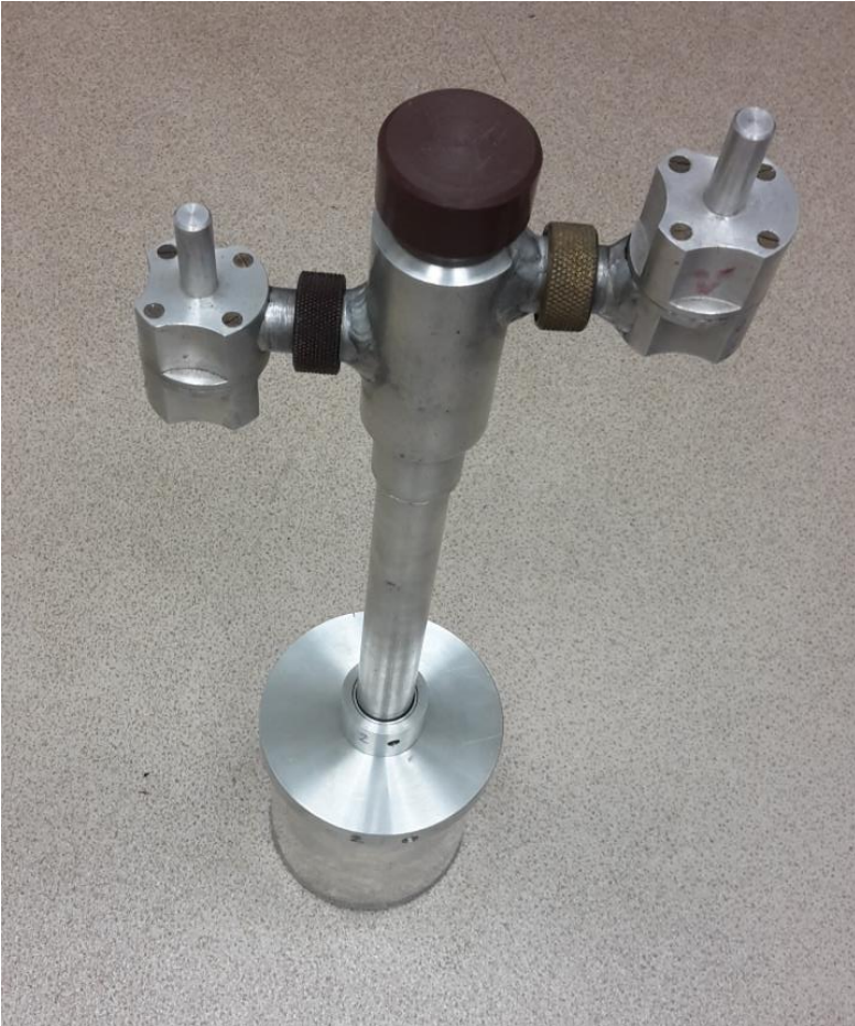
Irradiation Box for powder material "bulk" activation "foils" FLiBe, NaF, ... with Flexo-Rabbit ending
