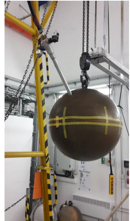
AF placement at the surface of Fe 50 cm On the left-top is Al Flexo-Rabbit ending
