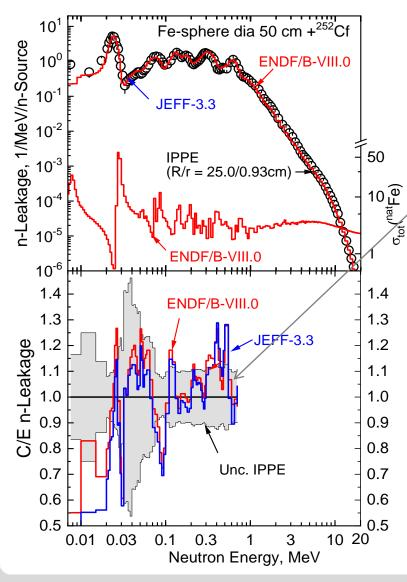
Neutron Leakage were measured by: - H proportional counter in 0.001 - 0.7 MeV - stilbene scintillator in 0.2 - 17. MeV and presented in ICSBEP as one n-spectrum
