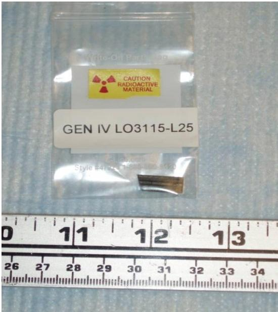
Measurements were made using unirradiated and irradiated nuclear graphite samples
