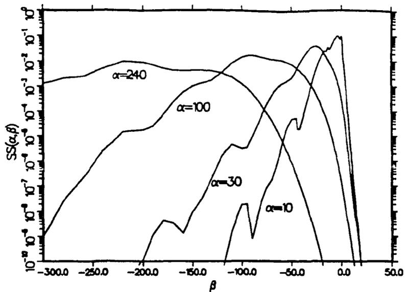
Figure 102: Script-S for liquid ortho deuterium at 19 K is shown as a function of  $\beta$  for several  $\alpha$  values, concentrating on high  $\alpha$  and  $\beta$  values.
