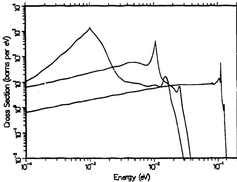
Figure 93: The spectra  $\sigma(E \rightarrow E')$  for liquid ortho hydrogen are shown for  $E = .001, .0106, \text{ and } .112 \text{ eV}$ .
