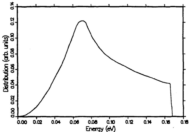
**Figure 42:** The frequency spectrum used for H in H<sub>2</sub>O. It is based on the original GA model converted to a uniform grid. Note that the right-hand limit is not vertical as in the original model.
