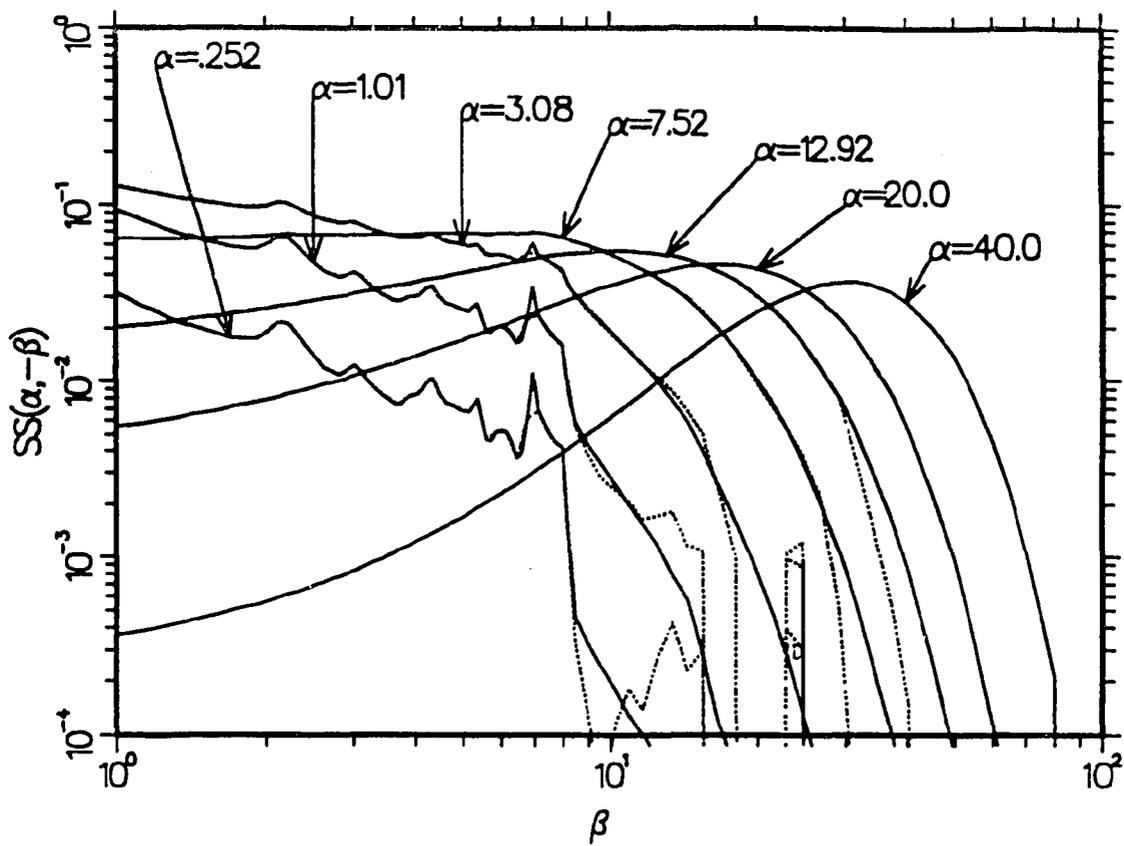
**Figure 32:** Asymmetric  $S(\alpha, -\beta)$  vs  $\beta$  for several  $\alpha$  values at a temperature of 296 K. The solid lines are the results of this calculation, and the dashed lines are for ENDF/B-VI.0.
