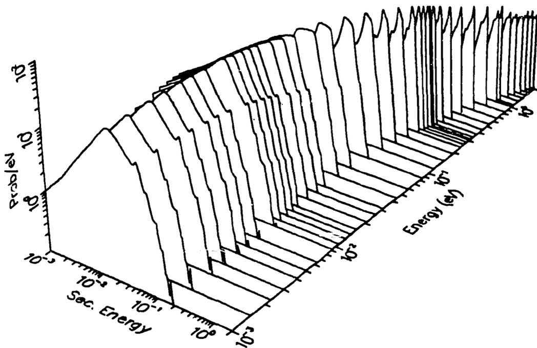
**Figure 41:** Perspective view of the spectra from thermal inelastic scattering on graphite at 296 K for energies up to 2 eV.
