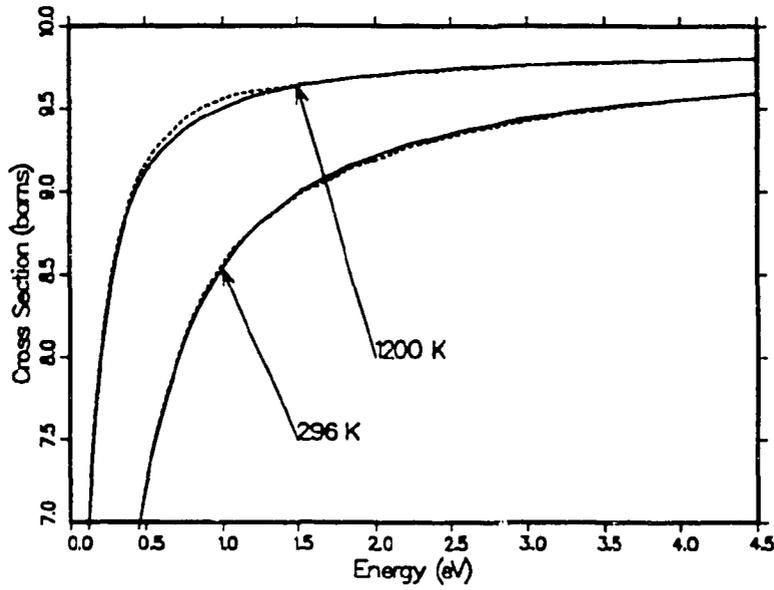
**Figure 23:** The inelastic cross section for BeO at temperatures of 296 K and 1200 K emphasizing the high-energy range. The dashed curves are for the ENDF/B-VI.0 evaluations.
