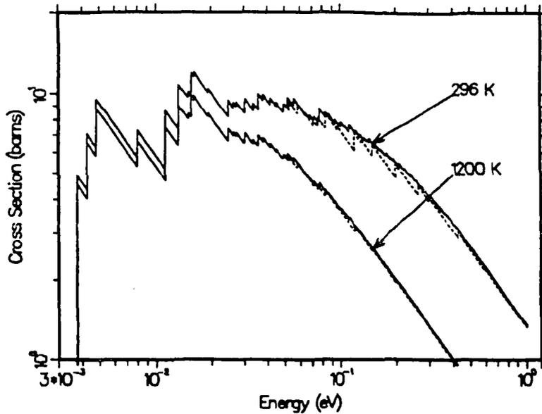
**Figure 24:** The coherent elastic cross section for BeO at temperatures of 296 K and 1200 K showing the Bragg peaks. The dashed curves are for the ENDF/B-VI.0 evaluations. Note the problem in the old evaluation near .1 eV for 296 K.
