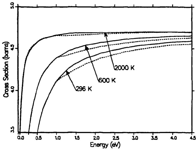
Figure 35: The incoherent inelastic cross section for graphite at temperatures from 296 K to 2000 K, emphasizing high energies. The old evaluation was designed to work to only 1 eV.
