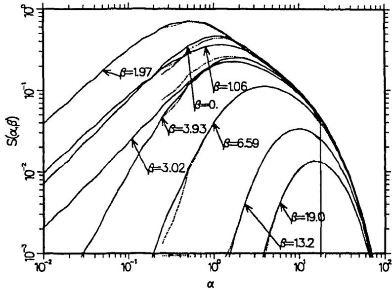
**Figure 4:**  $S(\alpha, \beta)$  vs  $\alpha$  for several  $\beta$  values at a temperature of 1200 K for Be. The solid lines are the results of this calculation, and the dashed lines are for ENDF/B-VI.0
