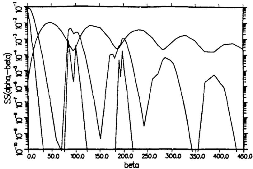
**Figure 73:**  $S(\alpha, -\beta)$  for solid methane shown as a function of  $\beta$  for the  $\alpha$  values 0.986 (lowest), 16.94, and 151.45 (highest). The four discrete levels show up as sharp triangles in the lowest curve. SS is used to denote script S.
