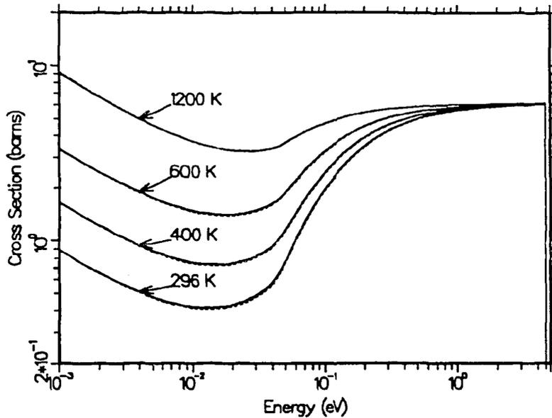
**Figure 10:** The inelastic cross section for Be at four temperatures emphasizing the low-energy range. The dashed curves are for the ENDF/B-VI.0 evaluations, and there is very little difference seen.
