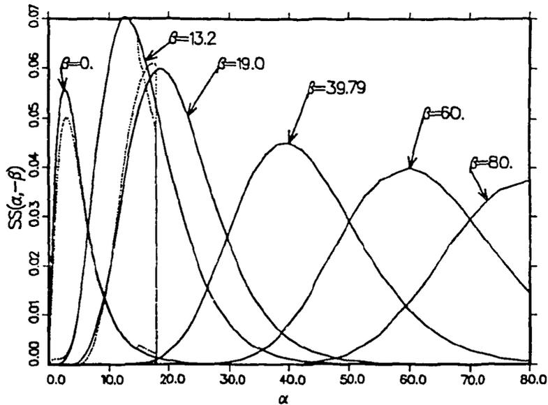
Figure 8:  $S(\alpha, -\beta)$  vs  $\alpha$  for several  $\beta$  values at a temperature of 296 K for Be. The solid lines are the results of this calculation, and the dashed lines are for ENDF/B-VI.0.
