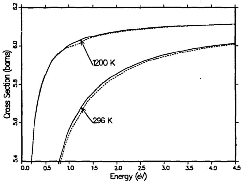
**Figure 11:** The inelastic cross section for Be at temperatures of 296 K and 1200 K emphasizing the high-energy range. The dashed curves are for the ENDF/B-VI.0 evaluations. Once again, little difference is seen.
