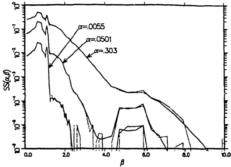
Figure 64:  $S(\alpha, -\beta)$  vs  $\beta$  for several  $\alpha$  values at a temperature of 296 K for Zr in ZrH. The solid lines are the results of this calculation, and the dashed lines are for ENDF/B-VI.0.
