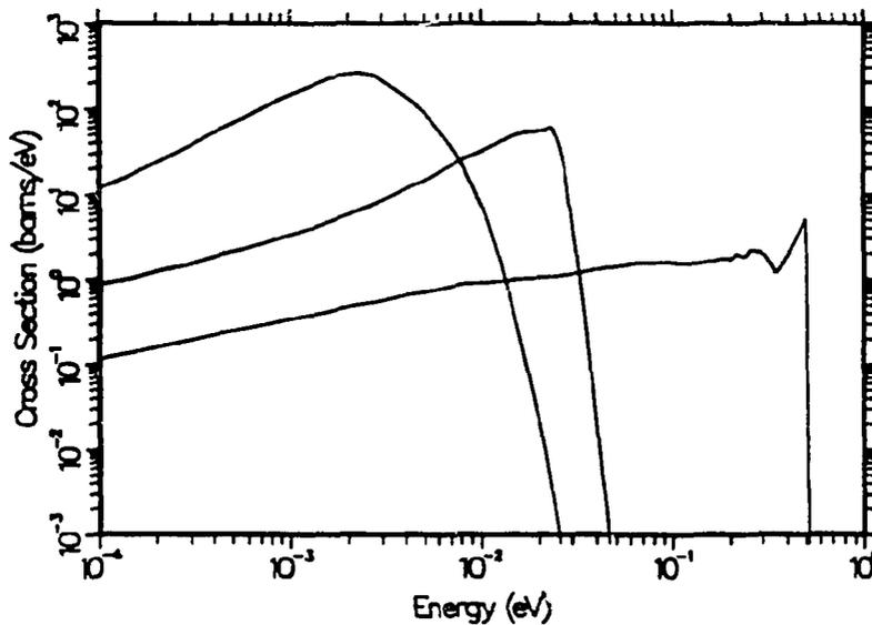
Figure 75: Neutron spectra  $\sigma(E \rightarrow E')$  for solid methane shown as functions of outgoing neutron energy  $E'$  for  $E = 0.0001, .0253, \text{ and } .503$  eV.
