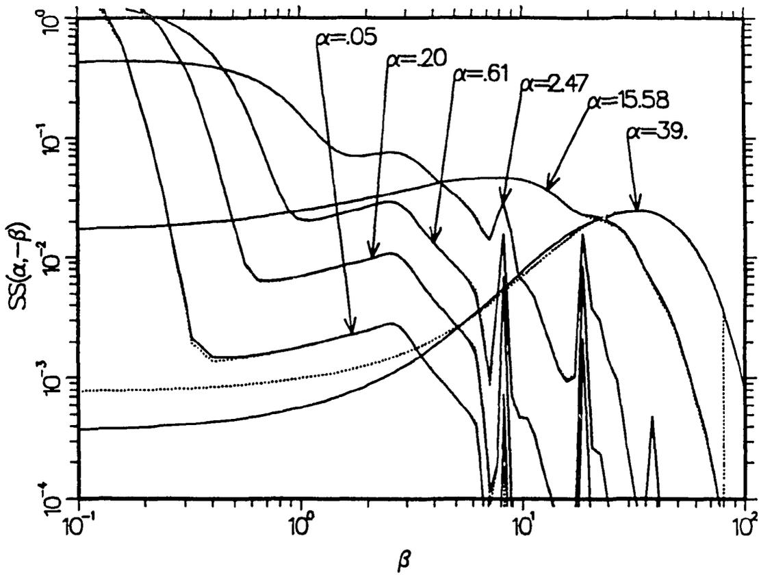
**Figure 43:**  $S(\alpha, -\beta)$  vs  $\beta$  for several  $\alpha$  values at a temperature of 296 K for H in  $H_2O$ . The solid lines are the results of this calculation, and the dashed lines are for ENDF/B-VI.0.
