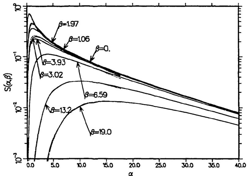
**Figure 5:**  $S(\alpha, \beta)$  vs  $\alpha$  for several  $\beta$  values of at a temperature of 1200 K for Be. The solid lines are the results of this calculation, and the dashed lines are for ENDF/B-VI.0. The effects of the new evaluation are similar to those seen at 296 K.
