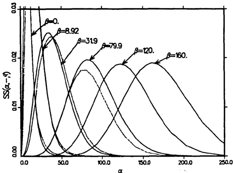
Figure 45:  $S(\alpha, -\beta)$  vs  $\alpha$  for several  $\beta$  values at a temperature of 296 K for H in  $H_2O$ . The solid lines are the results of this calculation, and the dashed lines are for ENDF/B-VI.0.
