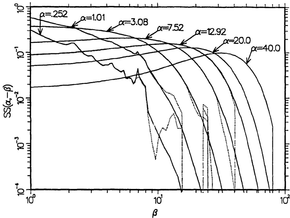
**Figure 33:** Asymmetric  $S(\alpha, -\beta)$  vs  $\beta$  for several  $\alpha$  values at a temperature of 1200 K. The solid lines are the results of this calculation, and the dashed lines are for ENDF/B-VI.0.
