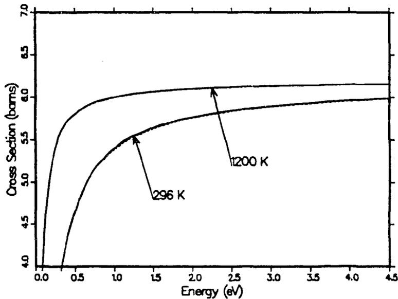
**Figure 67:** Expanded view of the integrated cross section for Zr in ZrH at the limiting values of the temperature. The solid lines are the results of this calculation, and the dashed lines are for ENDF/B-VI.0.
