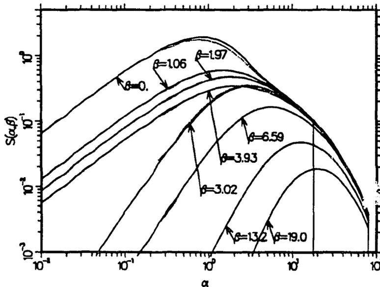
Figure 19:  $S(\alpha, \beta)$  vs  $\alpha$  for several  $\beta$  values in BeO at a temperature of 1200 K. The solid lines are the results of this calculation, and the dashed lines are for ENDF/B-VI.0. The effects of the new evaluation are similar to those seen at 296 K.
