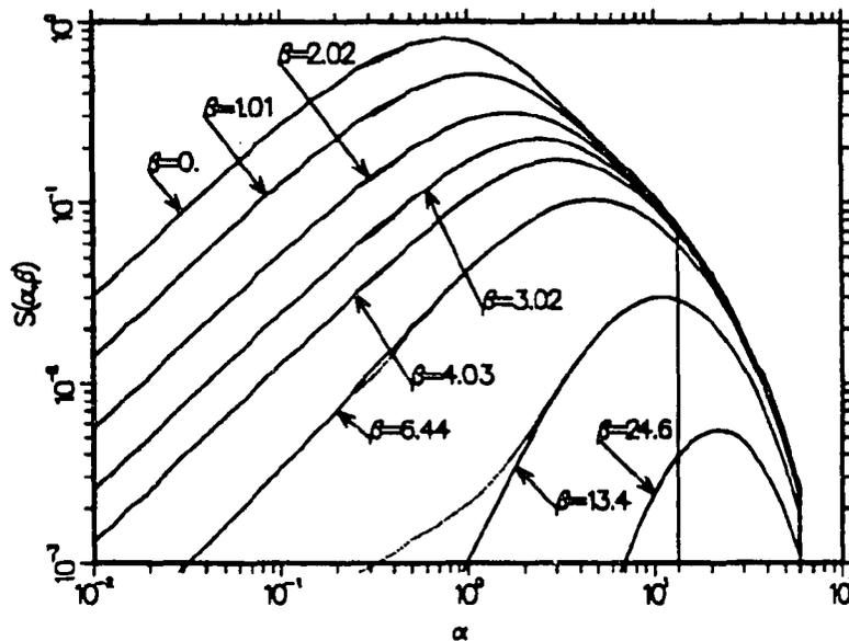
Figure 31:  $S(\alpha, \beta)$  vs  $\alpha$  for several  $\beta$  values at 1200 K. The solid lines are the results of this calculation, and the dashed lines are for ENDF/B-VI.0. Note that the dashed lines only cover the  $\alpha$  range from .25 to 13.4.
