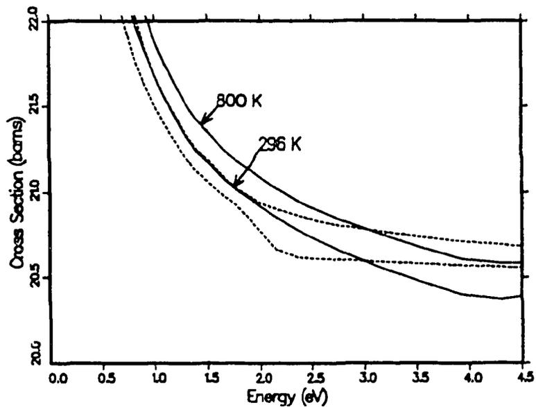
**Figure 47:** The inelastic cross section for H in H<sub>2</sub>O at temperatures of 296 K and 800 K emphasizing the high-energy range. The dashed curves are for the ENDF/B-VI.0 evaluations.
