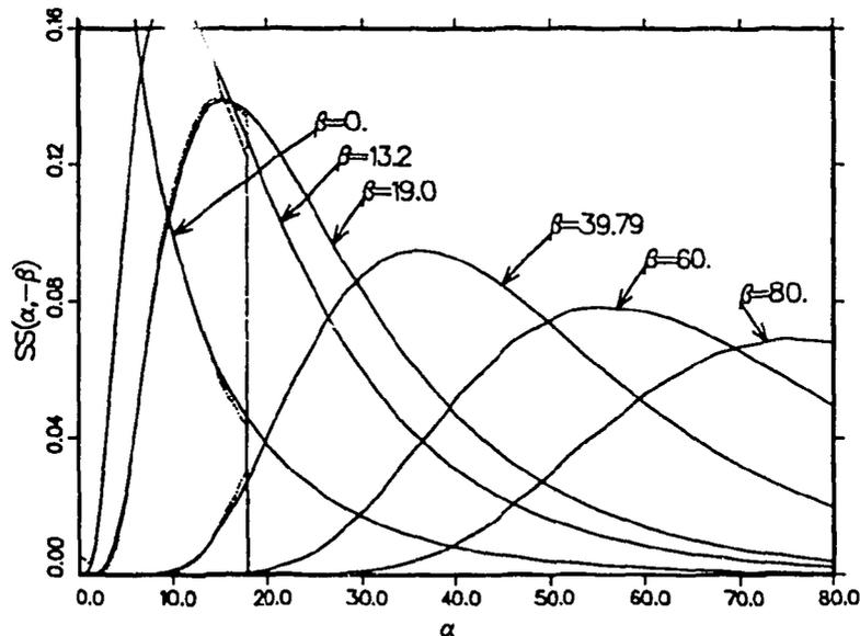
Figure 9:  $S(\alpha, -\beta)$  vs  $\alpha$  for several  $\beta$  values at a temperature of 1200 K for Be. The solid lines are the results of this calculation, and the dashed lines are for ENDF/B-VI.0.
