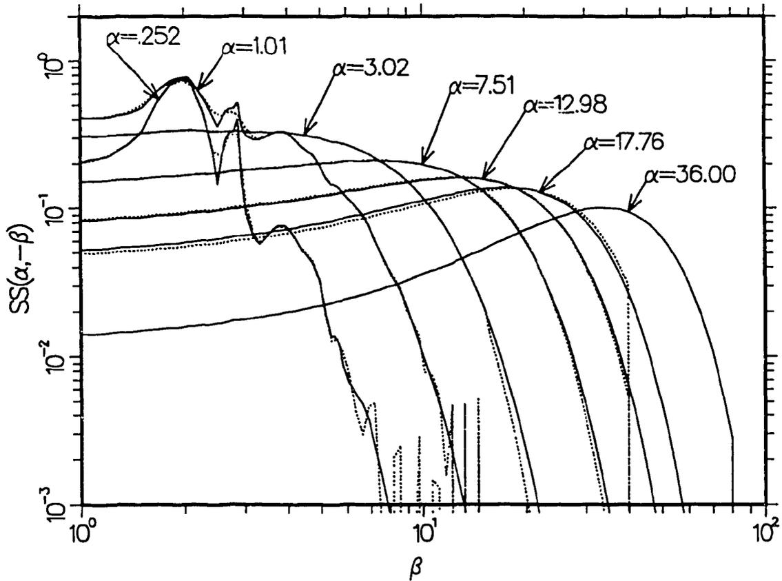
Figure 7:  $S(\alpha, -\beta)$  vs  $\beta$  for several  $\alpha$  values at a temperature of 1200 K for Be. The solid lines are the results of this calculation, and the dashed lines are for ENDF/B-VI.0. The comparisons show the same effects seen at 296 K, except the peaks and valleys are somewhat smoothed out at this high temperature.
