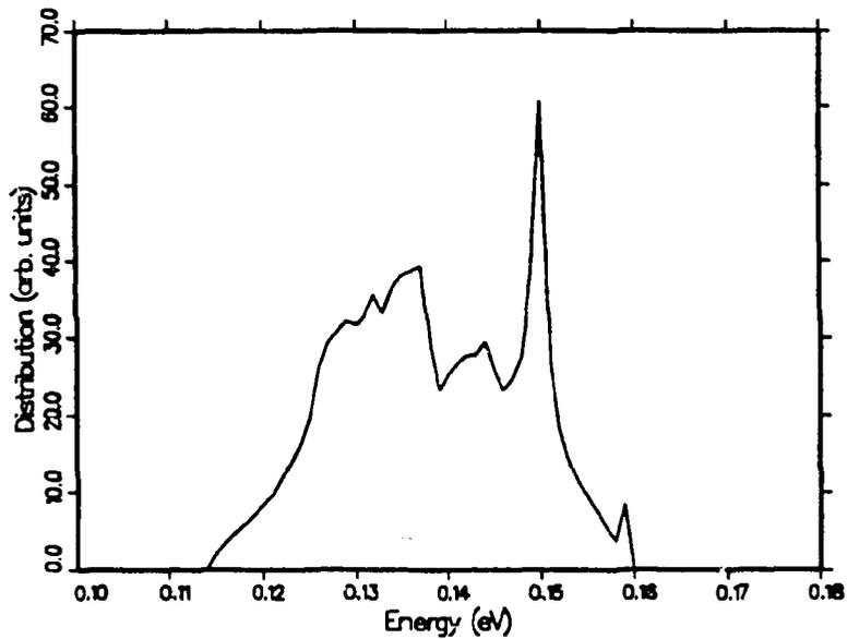
**Figure 53:** The frequency spectrum used for H in ZrH showing the optic modes. The function is zero between the top of the acoustic modes and the bottom of the optic modes.
