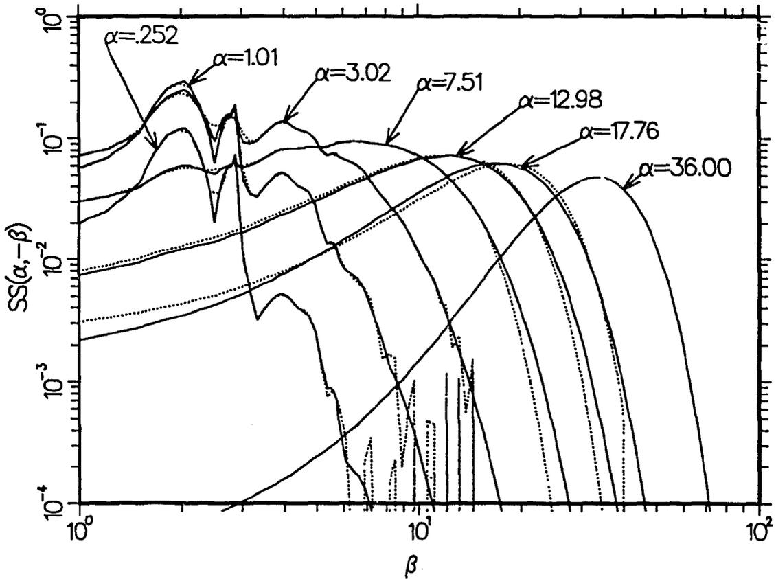
**Figure 6:**  $S(\alpha, -\beta)$  vs  $\beta$  for several  $\alpha$  values at a temperature of 296 K for Be. The solid lines are the results of this calculation, and the dashed lines are for ENDF/B-VI.0. The finer  $\beta$  grid used in the new evaluation does a better job of following the peaks and valleys resulting from features in  $\rho(\beta)$ . Also note that the new evaluation does a better job for small  $S$ . SS on the ordinate stands for script S.
