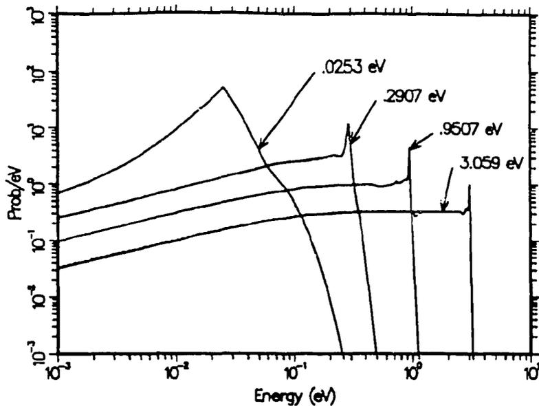
Figure 48: Secondary neutron spectra for H in H<sub>2</sub>O for several incident energies at a temperature of 296 K. The dashed curves are for the ENDF/B-VI.0 evaluation.
