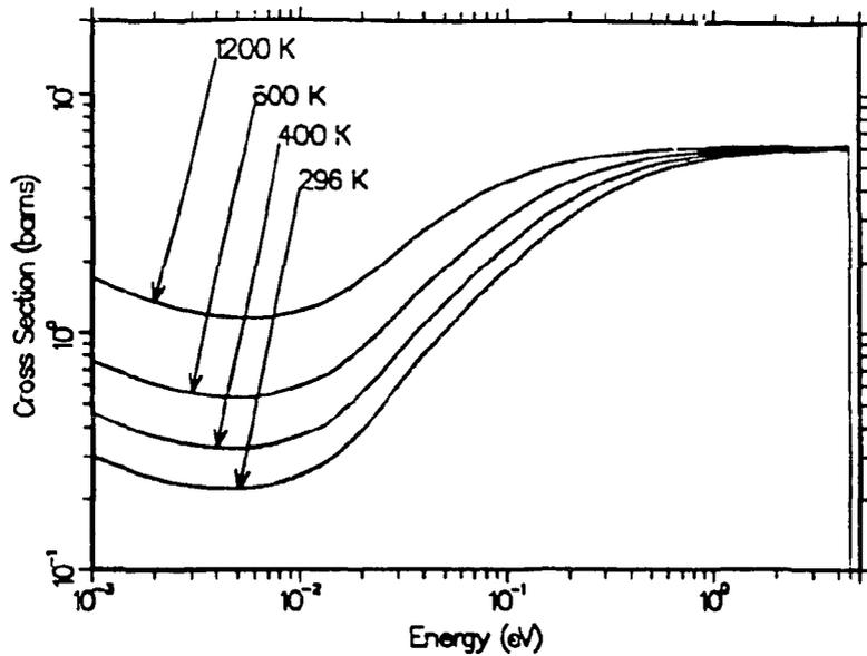
**Figure 66:** Integrated cross section for Zr in ZrH at four values of the temperature. The solid lines are the results of this calculation. The dashed lines for ENDF/B-VI.0 are almost completely hidden by the solid lines.
