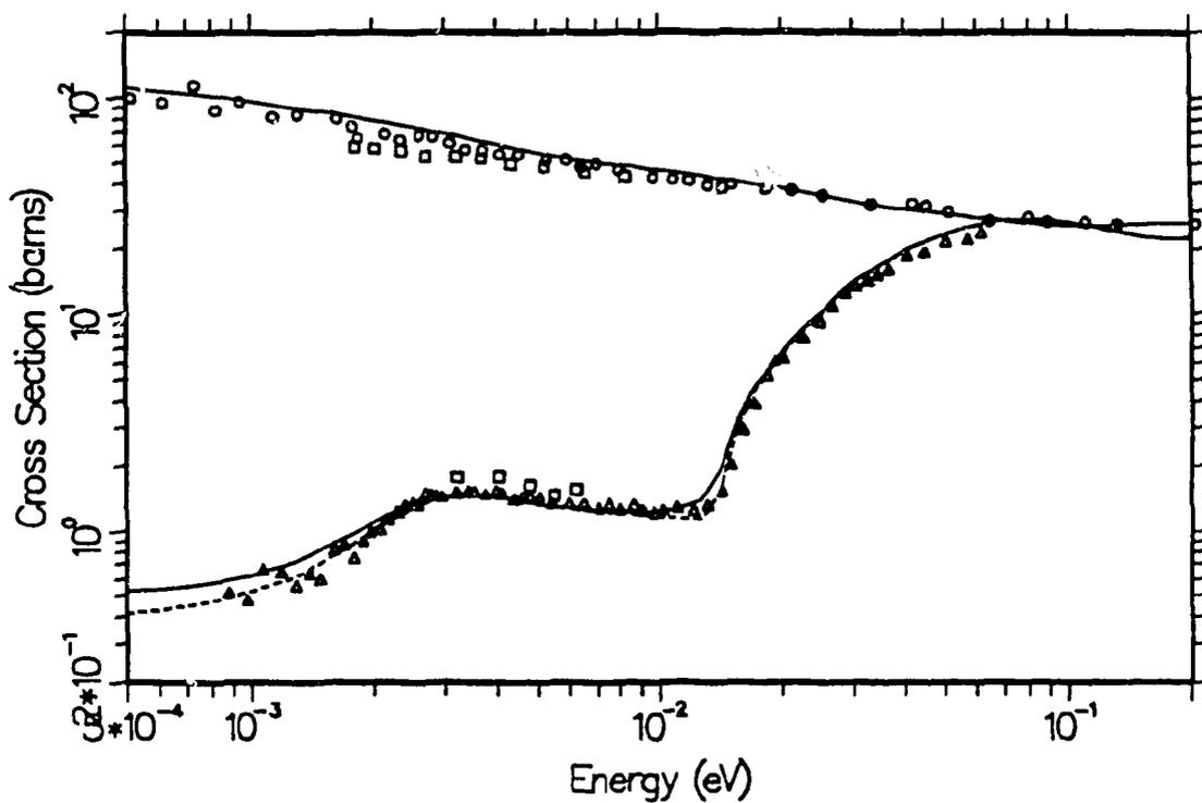
**Figure 91:** The cross sections for liquid ortho hydrogen (upper curve) and liquid para hydrogen (lower curve) are compared with experimental data (see Ref. 29) obtained by Squires (gas) at 20 K (squares), Whittemore at 20 K (circles), and Seiffert at 14 K (triangles). The solid curves are at 20 K, and the dashed curve is at 14 K. The sharp drop in the para cross section below 0.05 eV is due to spin coherence, and the second drop below .003 eV is due to intermolecular interference.
