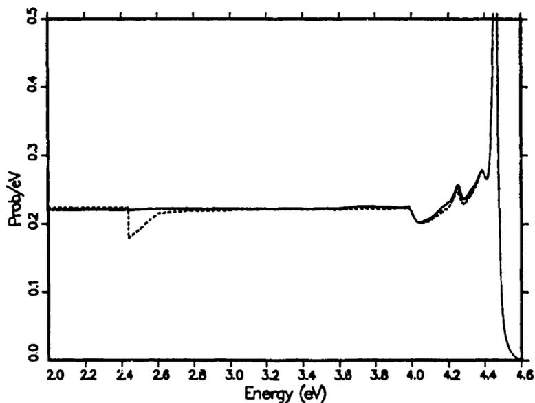
Figure 49: Expanded view of the secondary neutron spectrum at 4.46 eV for H in H<sub>2</sub>O at a temperature of 296 K. The dashed curve is the ENDF/B-VI.0 evaluation. The notch shows where the old evaluation used the SCT approximation.
