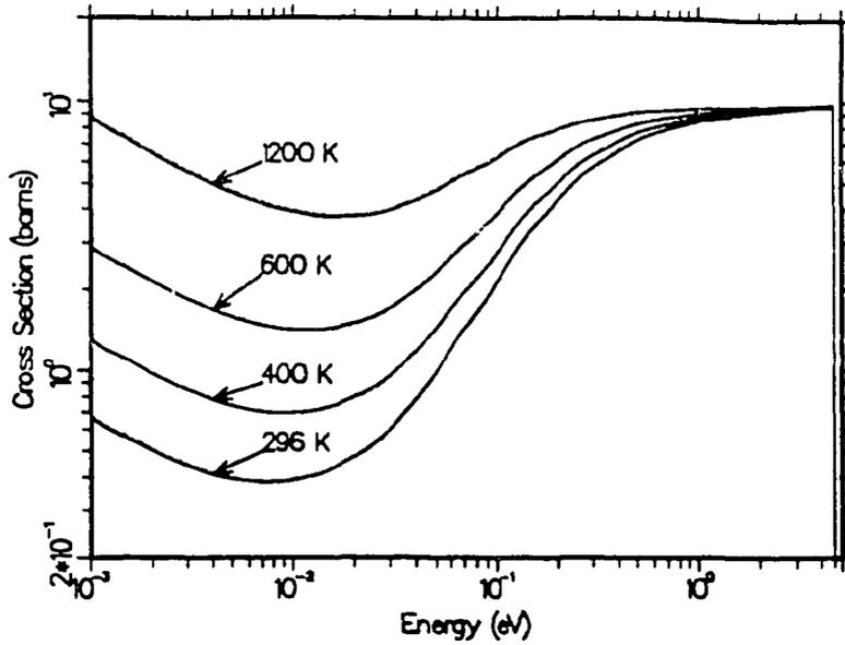
**Figure 22:** The inelastic cross section for BeO at four temperatures emphasizing the low-energy range. The dashed curves are for the ENDF/B-VI.0 evaluations, and there is very little difference seen.
