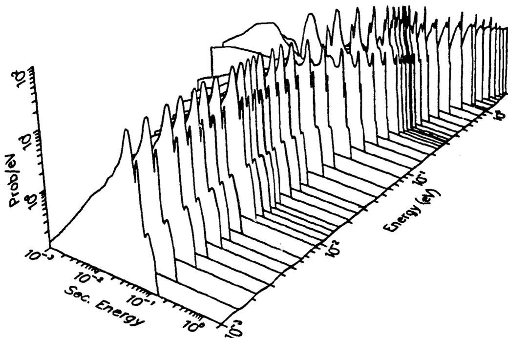
**Figure 16:** Perspective view of the secondary neutron spectra from thermal inelastic scattering from Be at 296 K for energies up to 2 eV.
