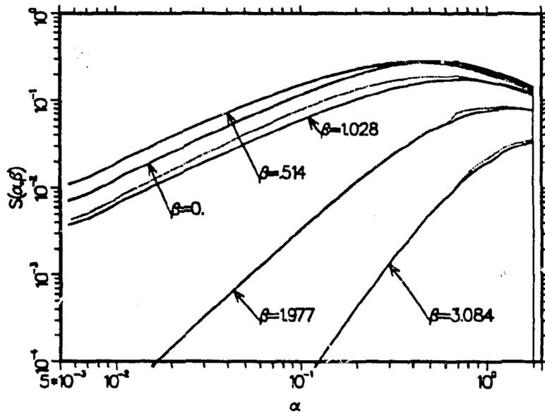
Figure 65:  $S(\alpha, \beta)$  vs  $\alpha$  for several  $\beta$  values at a temperature of 296 K for Zr in ZrH. The solid lines are the results of this calculation, and the dashed lines are for ENDF/B-VI.0.
