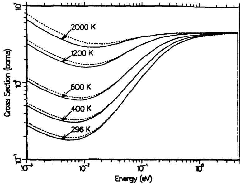
Figure 34: The incoherent inelastic cross section for graphite at temperatures from 296 K to 2000 K, emphasizing low energies.
