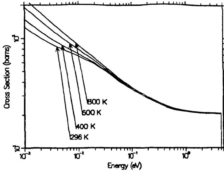
**Figure 46:** The inelastic cross section for H in H<sub>2</sub>O at four temperatures emphasizing the low-energy range. The dashed curves are for the ENDF/B-VI.0 evaluation.
