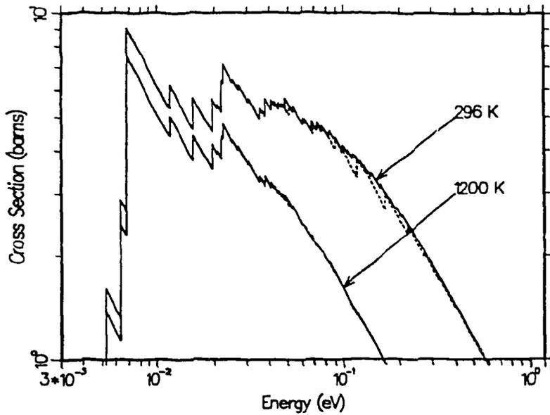
**Figure 12:** The coherent elastic cross section for Be at temperatures of 296 K and 1200 K showing the Bragg peaks. The dashed curves are for the ENDF/B-VI.0 evaluations. Note that the new evaluation fixes the problem in the old evaluation that is visible at 296 K for high energies.
