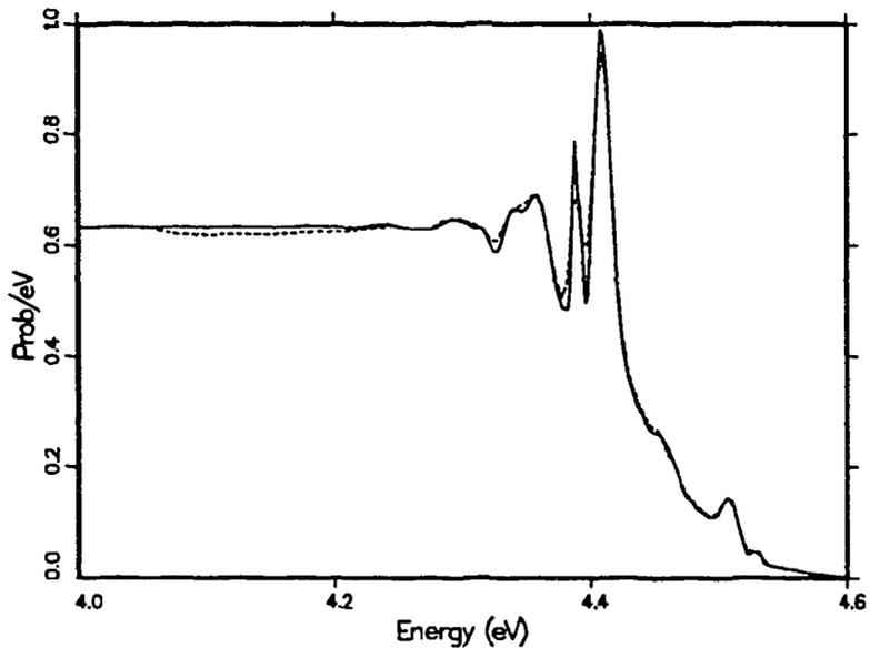
**Figure 15:** Expanded view of the secondary neutron spectrum at 4.46 eV for Be at a temperature of 296 K. The dashed curve is the ENDF/B-VI.0 evaluation. Note that the peaks and valleys are represented better in the new evaluation.
