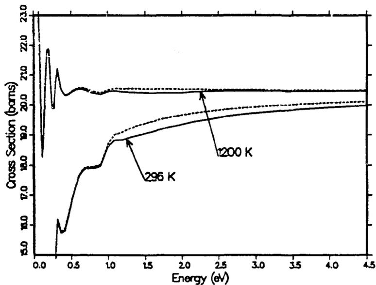
**Figure 57:** An expanded view of the integrated cross section for H in ZrH at the limiting values of the temperature. The solid curves are the new evaluation, and the dashed curves are from ENDF/B-VI.0. The differences above 1 eV are due to extending the  $\beta$  grid to cover energy transfers as large as 2 eV.
