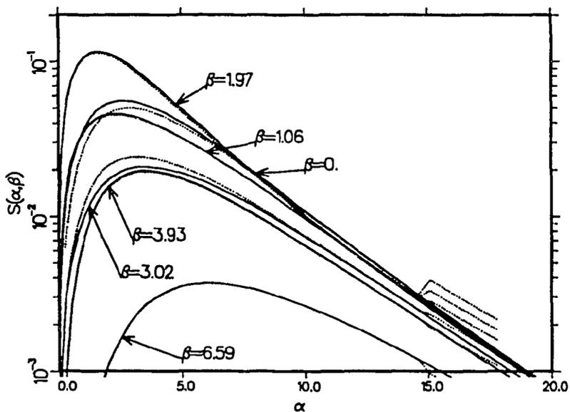
**Figure 3:**  $S(\alpha, \beta)$  vs  $\alpha$  for several  $\beta$  values at a temperature of 296 K for Be emphasizing the high- $\alpha$  side of the function. The solid lines are the results of this calculation, and the dashed lines are for ENDF/B-VI.0.
