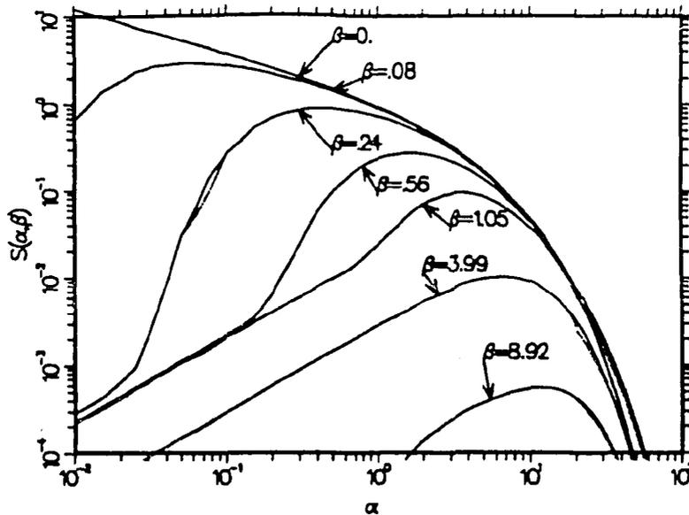
Figure 44:  $S(\alpha, \beta)$  vs  $\alpha$  for several  $\beta$  values at a temperature of 296 K for H in  $H_2O$  emphasizing the low- $\alpha$  side of the function. The solid lines are the results of this calculation, and the dashed lines are for ENDF/B-VI.0.
