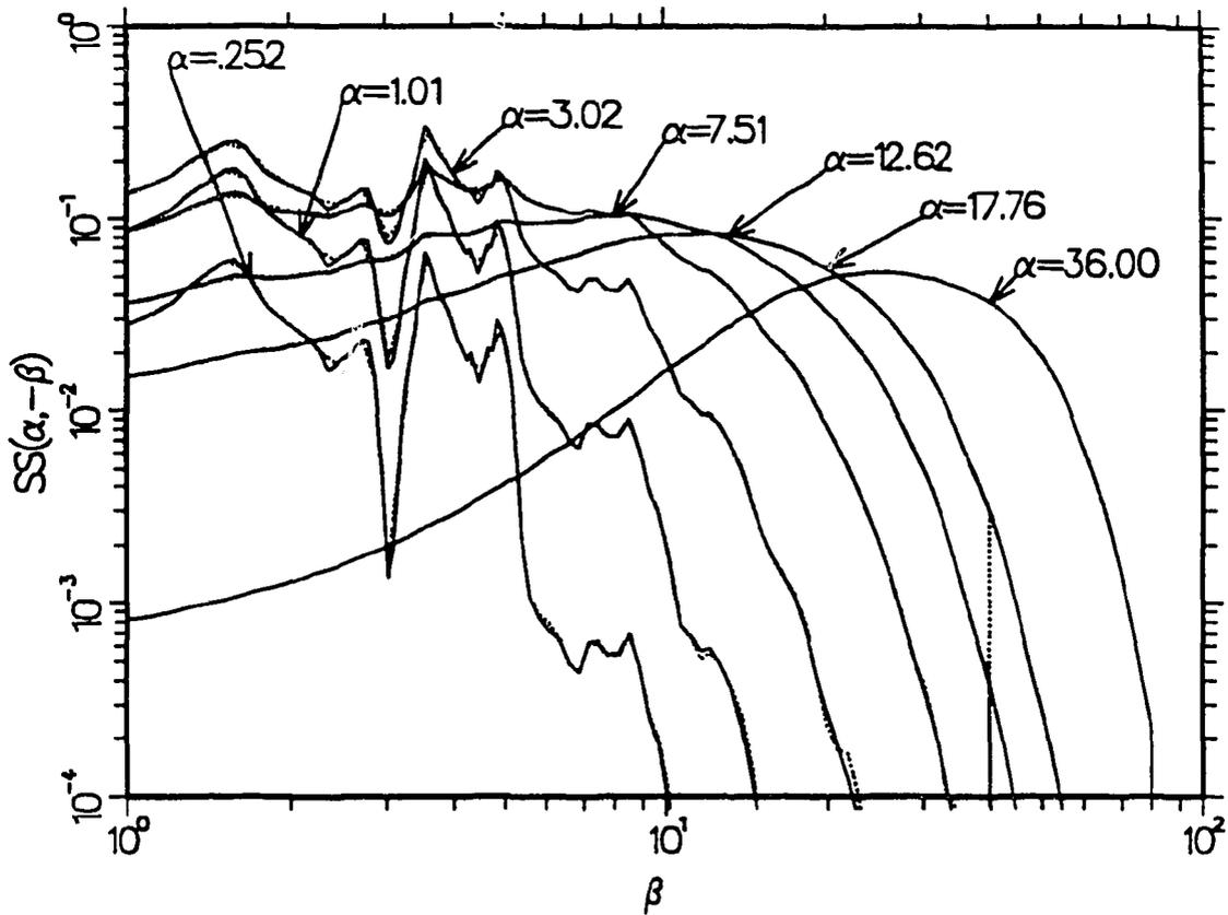
**Figure 20:**  $S(\alpha, -\beta)$  vs  $\beta$  for several  $\alpha$  values in BeO at a temperature of 296 K. The solid lines are the results of this calculation, and the dashed lines are for ENDF/B-VI.0. The finer  $\beta$  grid used in the new evaluation does a better job of following the peaks and valleys resulting from features in  $\rho(\beta)$ .
