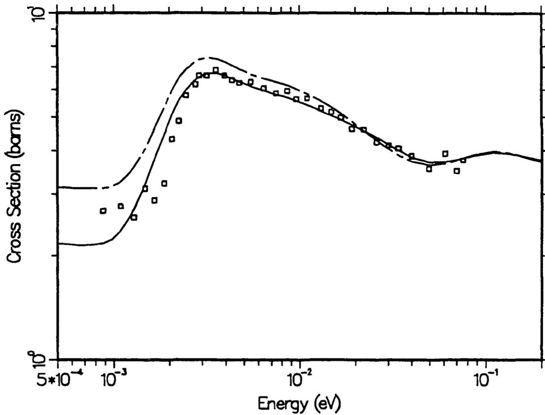
**Figure 104:** The cross sections for liquid para deuterium (solid curve) and liquid ortho deuterium (chain-dash curve) at 19 K are compared with experimental data of Seiffert for an equilibrium ortho-para mixture at 19 K (see Ref. 30). The drop in the cross sections below .003 eV is due to intermolecular interference.
