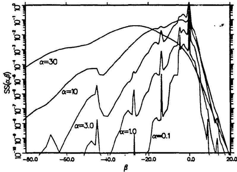
**Figure 101:** Script-S for liquid ortho deuterium at 19 K is shown as a function of  $\beta$  for several  $\alpha$  values, concentrating on the middle range of  $\alpha$  and  $\beta$  values.
