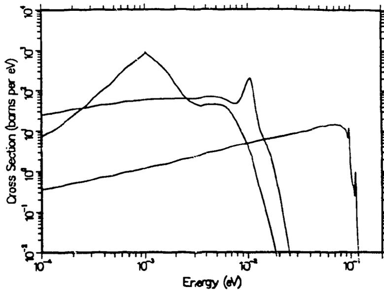
Figure 92: The spectra  $\sigma(E \rightarrow E')$  for liquid para hydrogen are shown for  $E = .001, .0106, \text{ and } .112 \text{ eV}$ .
