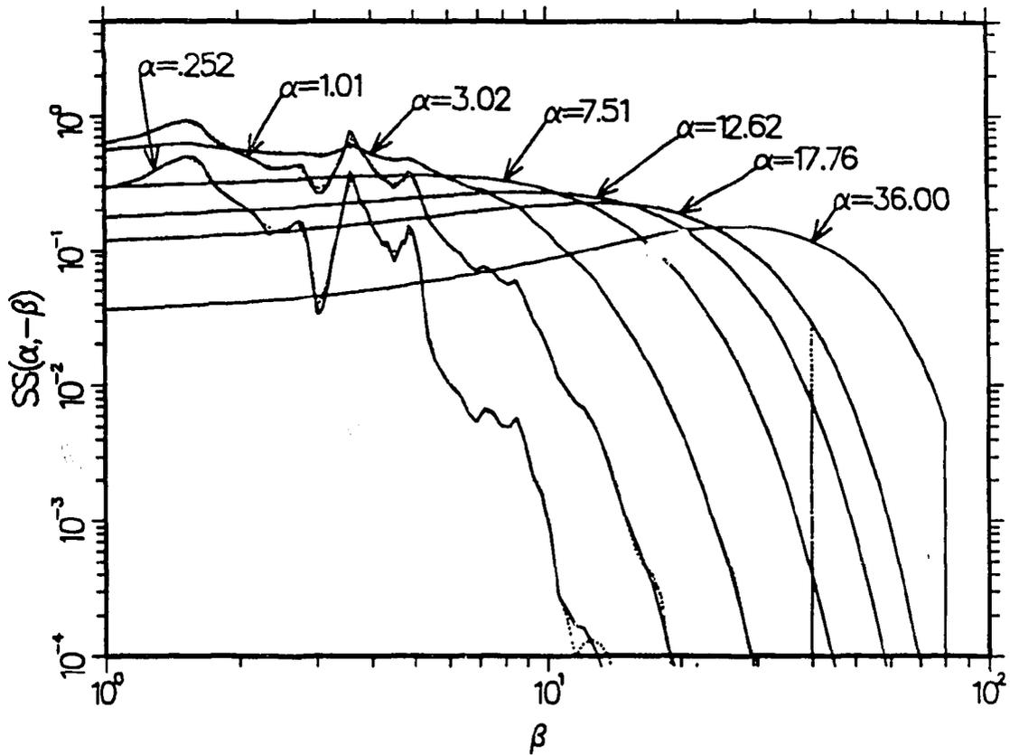
**Figure 21:**  $S(\alpha, -\beta)$  vs  $\beta$  for several  $\alpha$  values in BeO at a temperature of 1200 K. The solid lines are the results of this calculation, and the dashed lines are for ENDF/B-VI.0. The comparisons show the same effects seen at 296 K, except the peaks and valleys are somewhat smoothed out at this high temperature.
