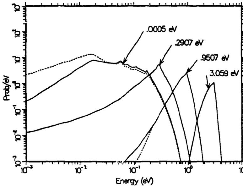
Figure 38: Spectra from thermal inelastic scattering from graphite at 1200 K for several incident energies.
