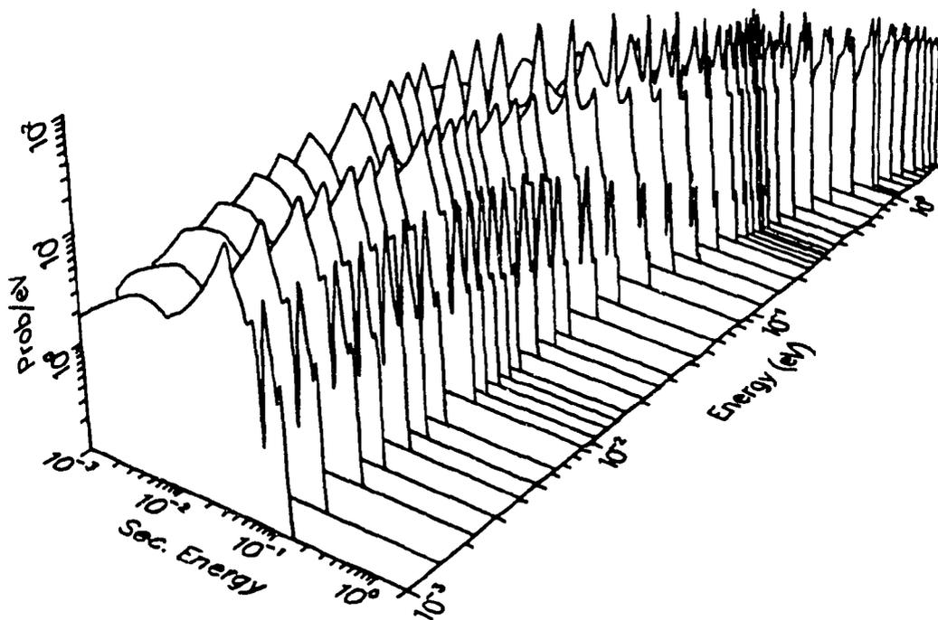
**Figure 28:** Perspective view of the secondary neutron spectra from thermal inelastic scattering from BeO at 296 K.
