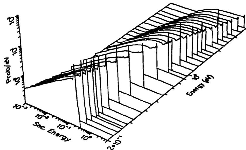
**Figure 51:** The isotropic component of the scattering from hydrogen bound in water for higher energies. Note that the results begin to converge to the free-gas shape except for some sharp features near  $E=E'$ . The variation in the size of the pseudo-elastic peak resulting from the free translation modes is an artifact of the plotting program.
