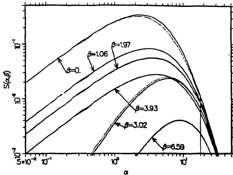
Figure 18:  $S(\alpha, \beta)$  vs  $\alpha$  for several  $\beta$  values in BeO at a temperature of 296 K emphasizing the low- $\alpha$  side of the function. The solid lines are the results of this calculation, and the dashed lines are for ENDF/B-VI.0.
