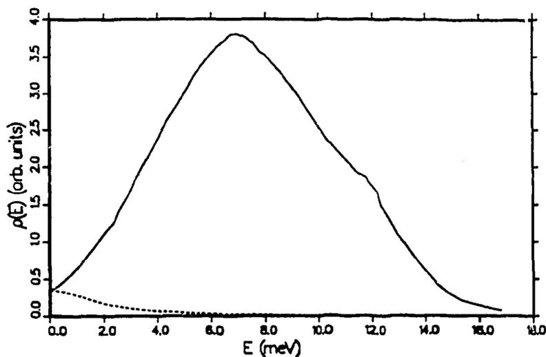
**Figure 76:** Frequency spectrum for liquid methane (solid) as given by Agrawal and Yip, including an analytic translational part (dashed) and a rotational part based on Gordon's analysis of the optical measurements of Ewing.
