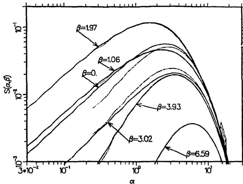
**Figure 2:**  $S(\alpha, \beta)$  vs  $\alpha$  for several  $\beta$  values at a temperature of 296 K for Be emphasizing the low- $\alpha$  side of the function. The solid lines are the results of this calculation, and the dashed lines are for ENDF/B-VI.0.
