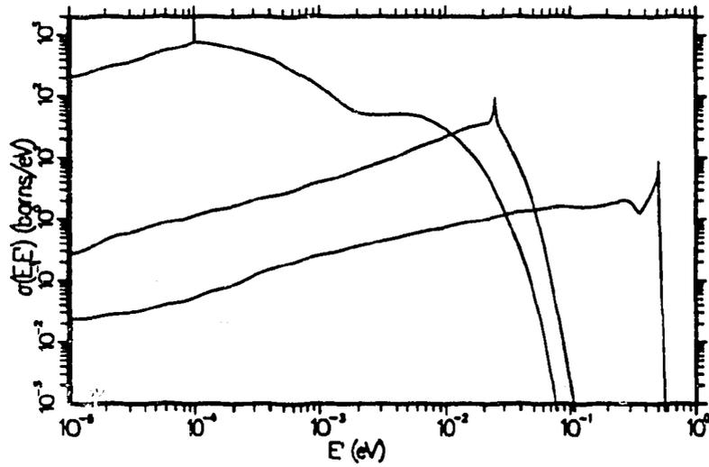
Figure 80: Neutron spectra  $\sigma(E \rightarrow E')$  are shown for  $E = .0001$ ,  $.0253$ , and  $.503$  meV. Note the sharp quasi-elastic peak that results from the diffusive term in the theory used here.
