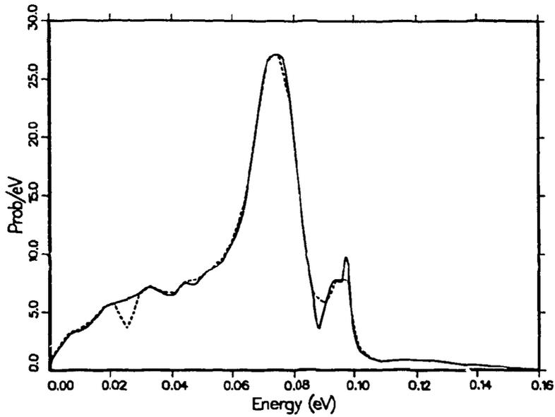
**Figure 14:** Expanded view of the secondary neutron spectrum at .0253 eV for Be at a temperature of 296 K. The dashed curve is the ENDF/B-VI.0 evaluation. The notch at .025 eV is due to a problem in the original frequency distribution.
