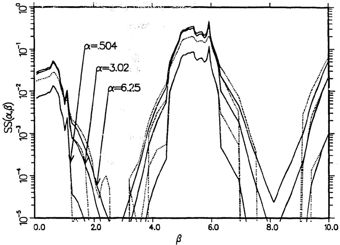
**Figure 54:**  $S(\alpha, -\beta)$  vs  $\beta$  for several  $\alpha$  values at a temperature of 296 K showing the low- $\beta$  side of the function. The solid lines are the results of this calculation, and the dashed lines are for ENDF/B-VI.0.
