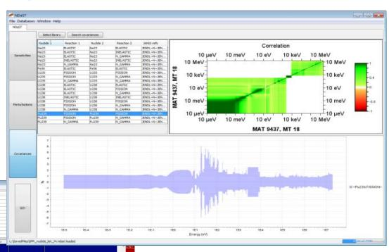
• In order that totals over different ranges of energy can be quickly computed and displayed, region selection bars may be used over the breakdown plot, which is colour-coded by magnitude.
